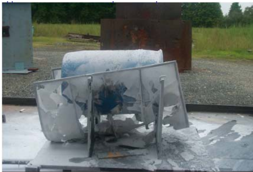
Figure 7. Post experiment photograph of 1.5 in. powder panel.
