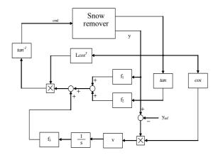
Figure 2. Integrated Servo System Control Block Diagram
