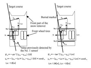
Figure 3. Lane Marker Sensor Guidance Method
