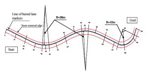
Figure 7. Layout of the Test Course
