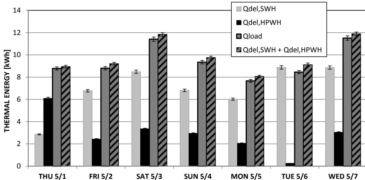
**Figure 2.** Daily thermal load provided by SWH and HPWH compared to the load delivered by overall system for the first week of May.
