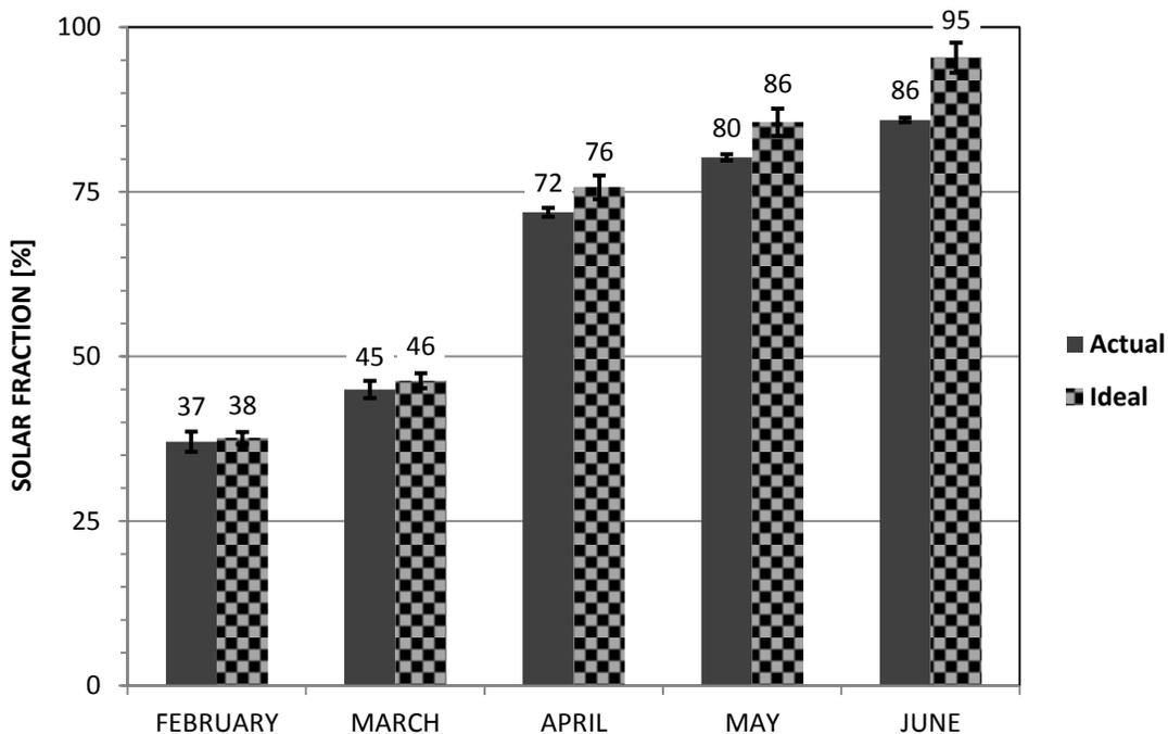
**Figure 4** Actual monthly SF versus ideal SF assuming no piping heat loss.
