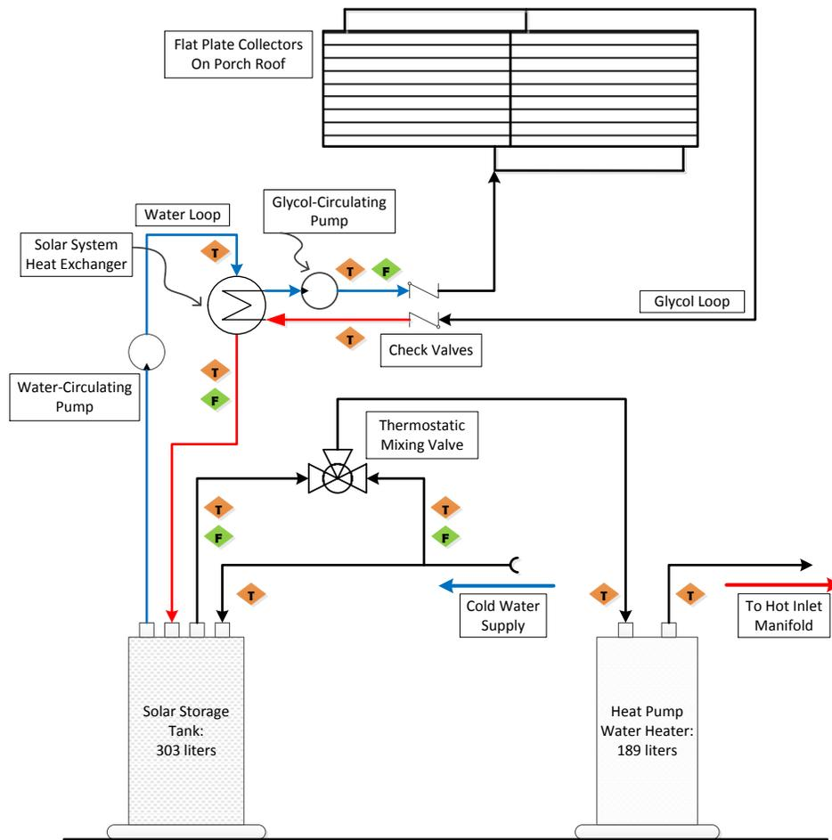
**Figure 1** Schematic of solar thermal and heat pump water heaters. Diamond symbols with “T” indicate temperature measurement locations in the stream of fluid flow and diamond symbols with “F” show flow measurement locations.
