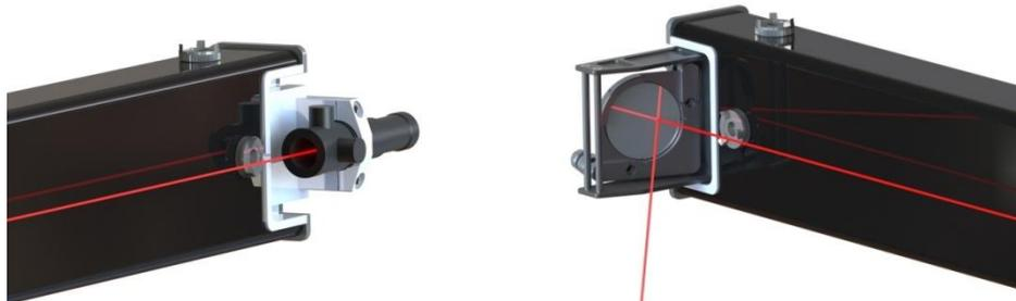
**Figure 5. Detailed View of Alignment Laser and Folding Mirror**
