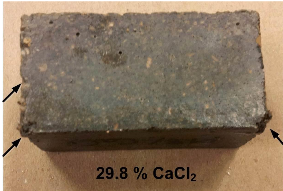
Figure 8 - Damage at the edges of mortar specimens immersed in a 29.8 % \text{CaCl}_2 solution prior to the AE-LGCC experiment (arrows highlight the damage and degradation).
