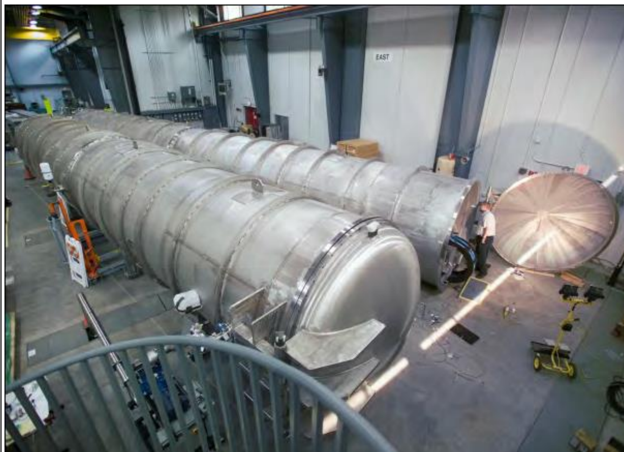
Figure 3: Detector tanks for two SANS instruments at the HFIR. The General Purpose SANS (with tank door open) and the bioSANS (nearer) are shown. The sample positions are at the other end of the tanks (far left).
