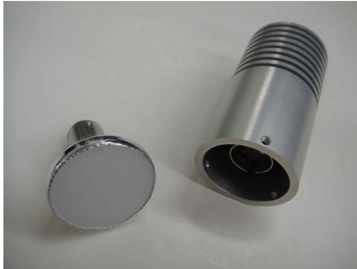
Figure 1 – Photograph of the 2\pi TSRF transfer standard lamp and its lamp housing
