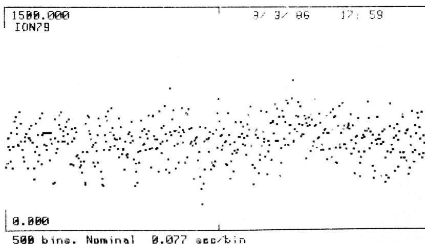
**Fig. 6.** Sequence of 194 nm  $\text{Hg}^+$  fluorescence photocounts of duration 77 ms. Frequency of laser is fixed and detuned further below resonance, compared to Fig. 5. The horizontal and vertical scales are the same as in Fig. 5.
