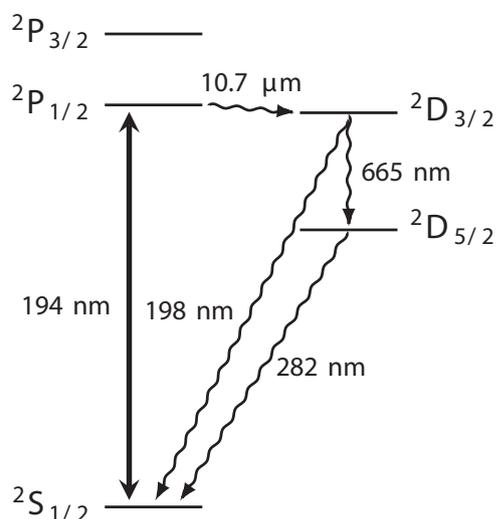
**Fig. 3.** Energy-level diagram of the Hg<sup>+</sup> ion and radiative decays relevant to the NIST experiment with only the 194 nm laser applied.
