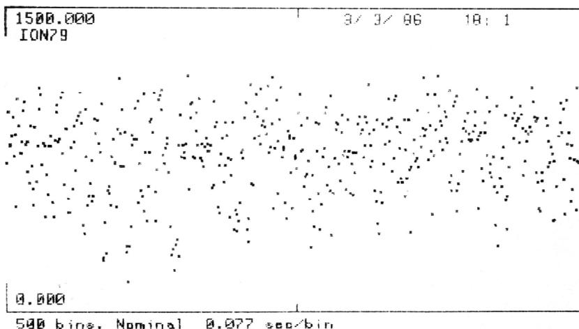
**Fig. 5.** Sequence of 194 nm  $\text{Hg}^+$  fluorescence measurements of duration 77 ms. Vertical scale limits are 0 and 11.55 counts per bin. Frequency of laser is fixed and close to resonance. Measurement time increases from left to right. The lowest-fluorescence measurements represent periods when the ion spent much of the time in a metastable state. No background has been subtracted from the data.
