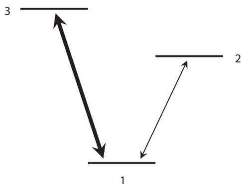
**Fig. 1.** Energy-level diagram of a three-level atom suitable for 'shelved-electron detection' and observation of 'macroscopic quantum jumps.' The  $1 \leftrightarrow 3$  transition is 'strong,' while the  $1 \leftrightarrow 2$  transition is 'weak.'
