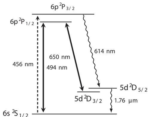
Fig. 8. Energy-level diagram of  $\text{Ba}^+$ , showing the levels and transitions involved in the experiments of the University of Washington and University of Hamburg groups.
