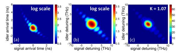
FIG. 2. (Color online) Joint probability distribution, integrated for 2 min (a) as measured, log-scale plot of the raw joint time-of-arrival probability distribution, (b) log-scale plot of the joint-spectral intensity (JSI), (c) absolute value of the joint-spectral amplitude (JSA) distribution.
