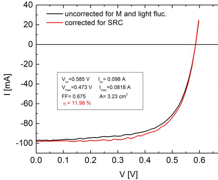
Fig. 9. (a)  $I$ - $V$  curves for a solar cell before and after correction of the raw measurement to standard reporting conditions. The reason for the noise in the data is related to the short term fluctuations in the lamp's intensity profile.
