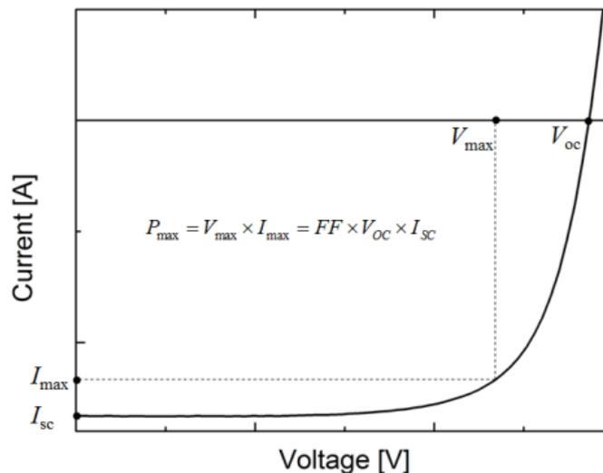
Fig1. A generic  $I$ - $V$  curve of a solar cell under sun illumination.
