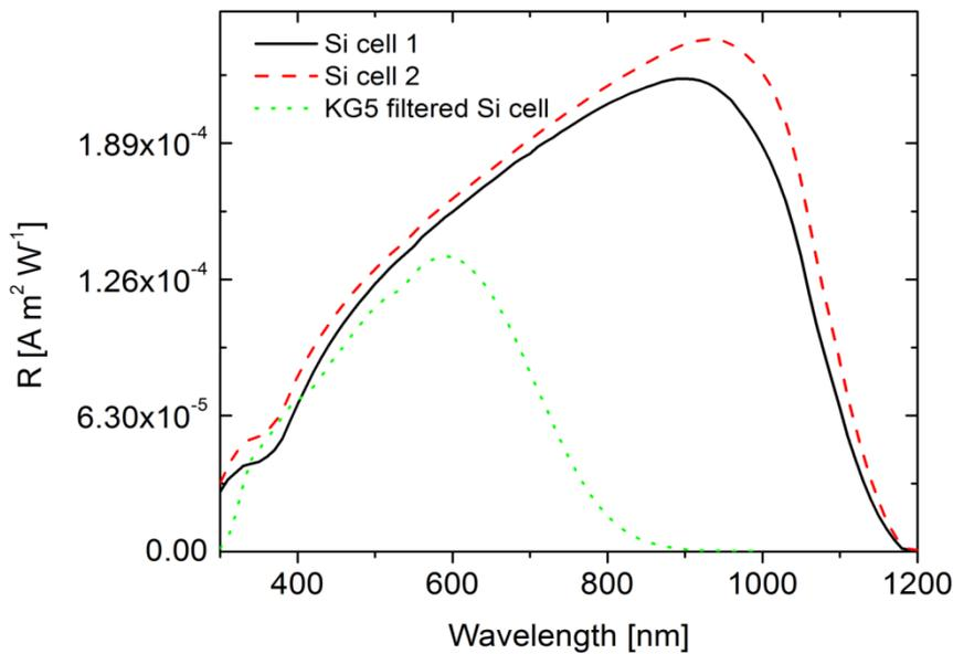
Fig. 6. Irradiance mode spectral response curves of a few solar cells.
