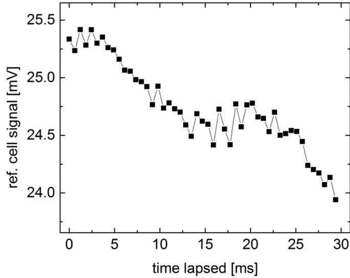
Fig. 3. The temporal stability of a flash solar simulator during the course of a 30 ms  $I$ - $V$  measurement.
