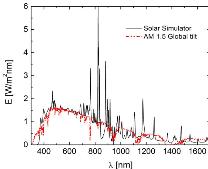
Fig. 2. The irradiance spectrum of a Xe flash solar simulator. For comparison, the AM 1.5 G spectrum is also plotted.
