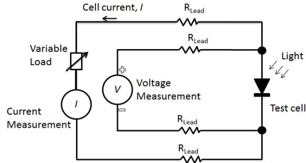
Fig 7. 4 wire  $I$ - $V$  measurement schematic
