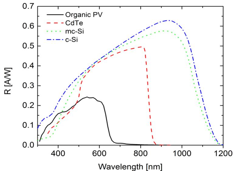
Fig. 5. Power mode spectral response curves of a few different types of solar cells.
