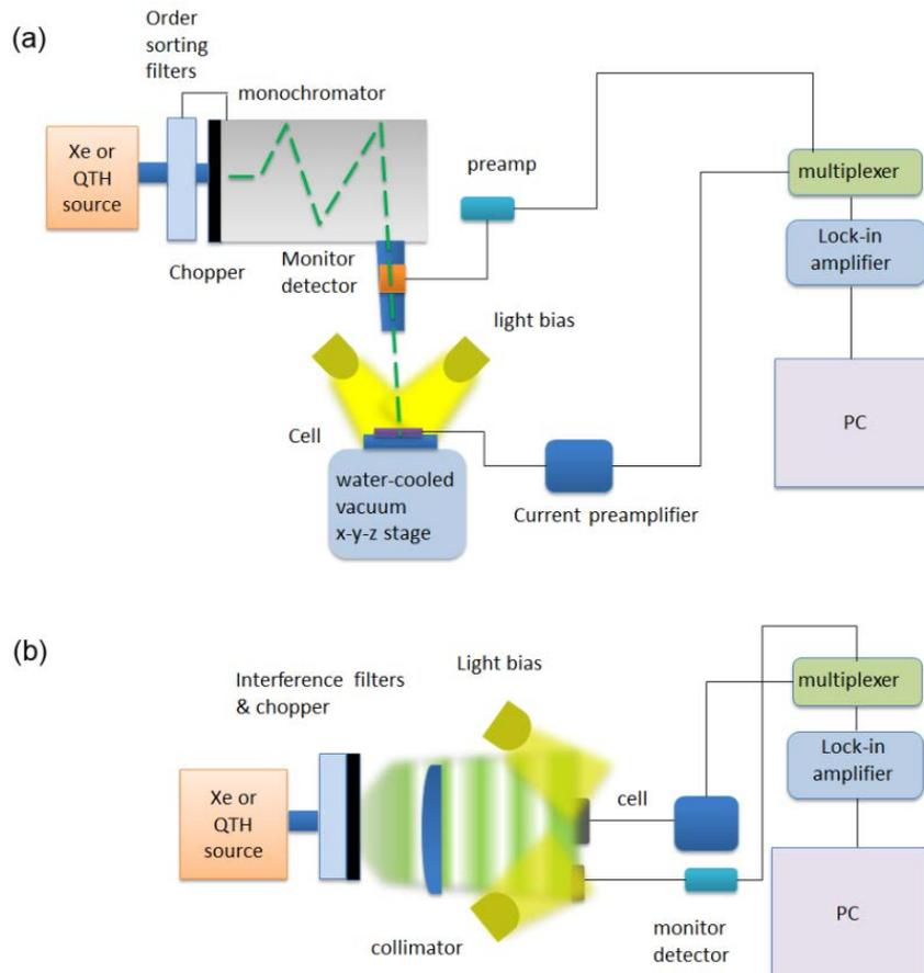
Fig 4. (a) Schematics of a monochromator-based SR measurement system where the probe beam underfills the cell. (b) An example of an SR measurement system where the beam overfills the cell.
