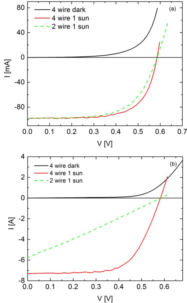
Fig. 8. (a) Comparison between 2 wire and 4 wire  $I$ - $V$  measurements on a small 4 cm<sup>2</sup> solar cell. (b) Same comparison on a larger cell with an area of 219 cm<sup>2</sup>. The  $I$ - $V$  curves measured in the dark are also plotted for both solar cells.
