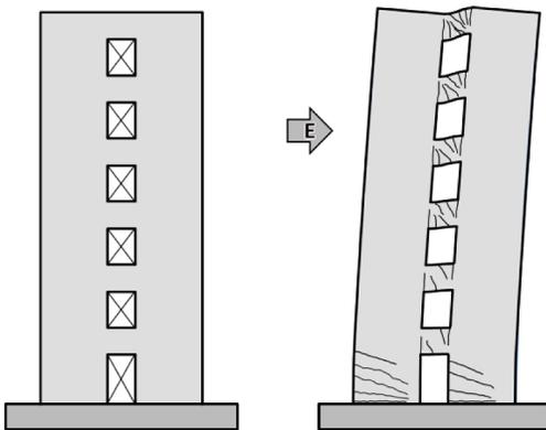
Figure 2-9 – Coupled wall geometry and target yield mechanism.
