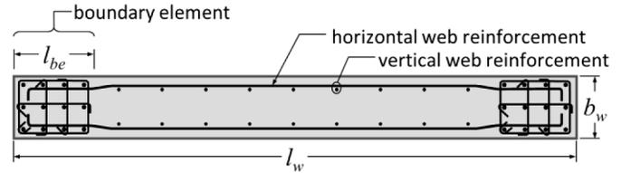
Figure 2-10 – Typical reinforcement for rectangular wall.
