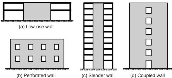
Figure 2-1 – Some illustrative structural wall elevations.
