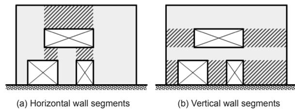
Figure 2-8 – Vertical and horizontal wall segments (hatched).
