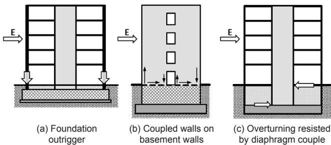
Figure 2-6 – Various ways to spread overturning resistance.
