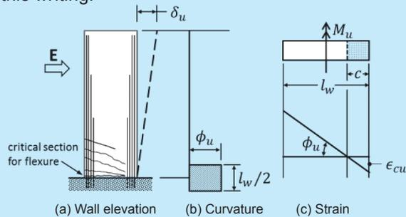
Figure 5-7 – Model to determine confinement trigger.
