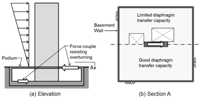
Figure 2-5 – Force transfers between walls and diaphragms.
