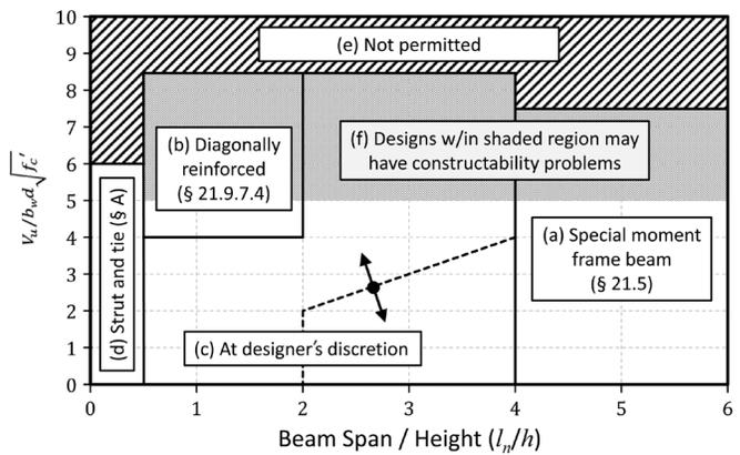
**Figure 5-11** – Seismic coupling beam design space.
