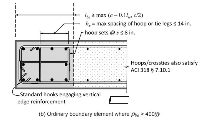
**Figure 5-3** – Special and ordinary boundary elements.
