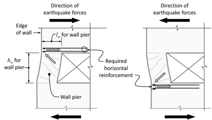
Figure 5-10 – Reinforcement required above and below wall pier.
