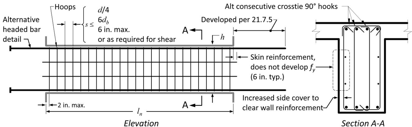
**Figure 5-12** – Details for conventionally reinforced coupling beams.
