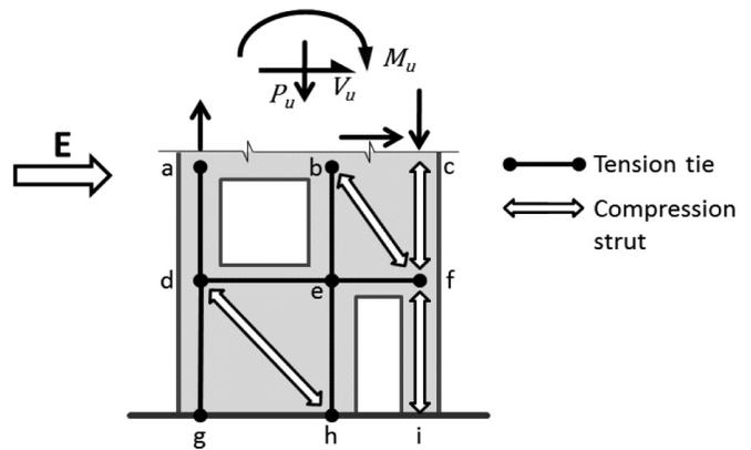
**Figure 5-20**– Strut-and-tie model.
