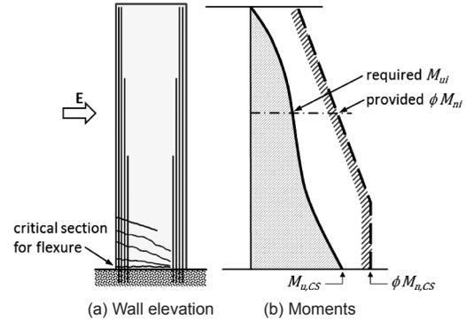
**Figure 3-1** – Provided versus required flexural strength in a wall with a single critical section.
