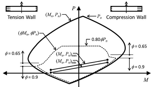
Figure 5-17 –  $P$ - $M$  capacity check for coupled walls.
