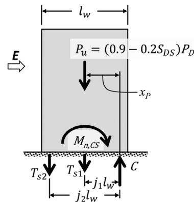
Note: This is a model showing forces to be considered for estimation of design tension forces  $T_{s1}$  and  $T_{s2}$  for wall without coupling.
