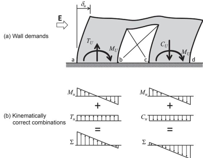
Figure 5-8 – Elevation of laterally displaced coupled wall system.
