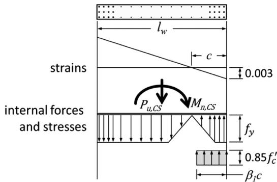
**Figure 5-4** – Calculation of neutral axis depth  $c$ .
