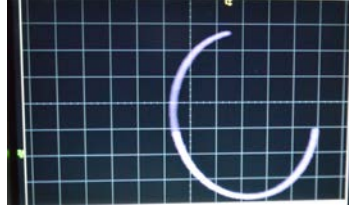
Figure 7b Photo-detector signals plotted as x - y, no modulation
