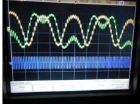
Figure 7a Photo-detector signals in quadrature with 1 kHz modulation on reference mirror.
