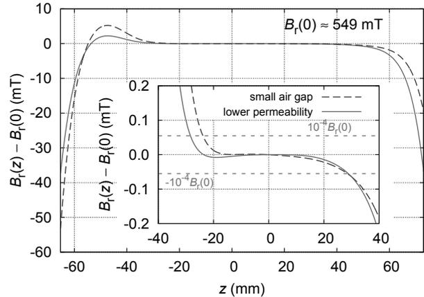
Fig. 3. The radial flux density as a function of vertical position. The inset shows the central region magnified such that the total size of the vertical axis extends  $\pm 4 \times 10^{-4}$  around the value at  $z = 0$ . Two shimming methods lead to a similar profile: introducing a small air gap (dashed line) and reducing the relative permeability of the iron (solid lines).
