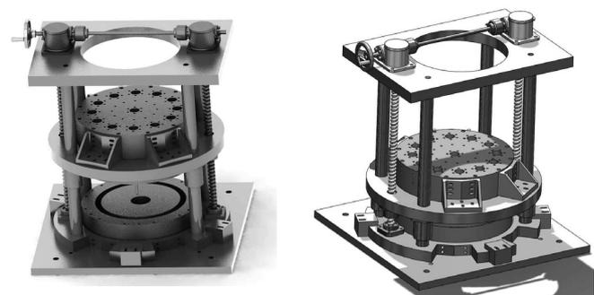
Fig. 1. To install the the coil in the magnet, it can be split open such that the top two thirds of the magnet separate from the bottom third. On the left: magnet in the magnet-splitter with the magnet in the open state. On the right: magnet in the magnet-splitter in the closed state.
