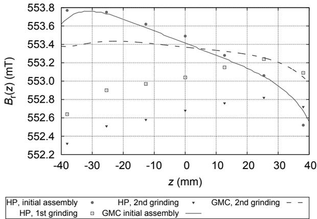
Fig. 2. The points represent data measured with the EEC Hall probe (HP) after initial assembly, the first, and second grinding process. Lines indicate measurements performed with the gradiometer coil (GMC) after initial assembly and after the second grinding. The gradiometer coil readings are 4.2 mT higher. For this plot 4.2 mT were subtracted from the measurements performed with the gradiometer coil.
