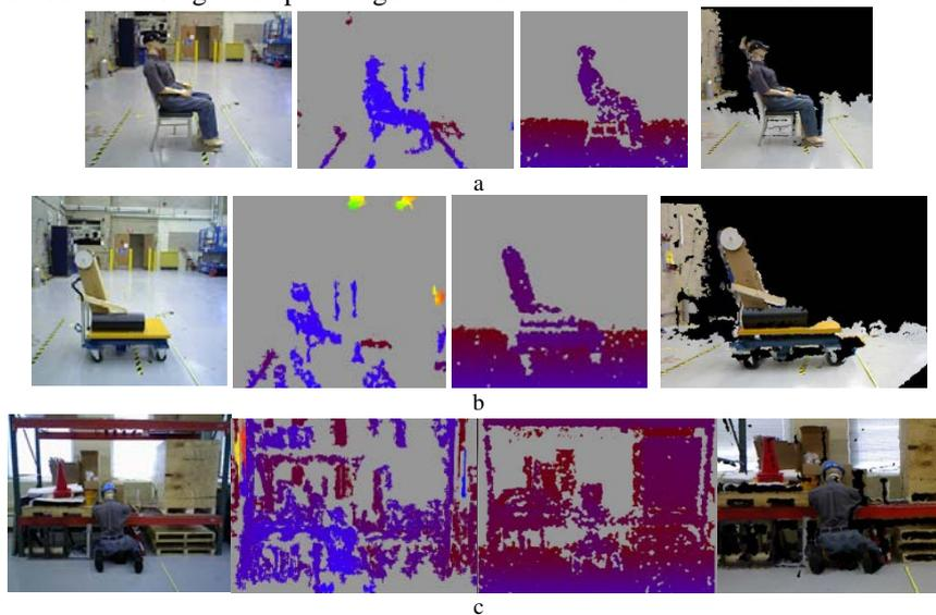
Figure 5 – (left to right) Xtion/Kinect color data, stereo depth data, Xtion/Kinect depth, and Xtion/Kinect fused color and depth data of (a) a seated mannequin, (b) mocked materials, and (c) a crouched worker in front of industrial shelving.
