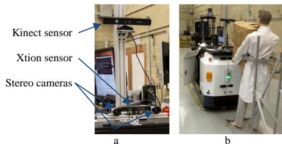
Figure 4 - Photos of the (a) sensors and (b) AGV used for testing. In (b), the AGV was moving towards the mannequin for dynamic data collection purposes.
