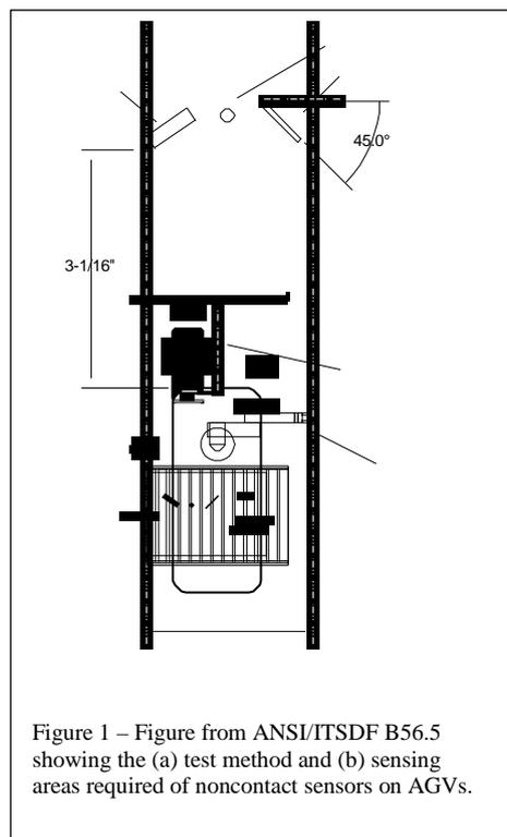
the test piece placement for the noncontact sensing as defined in the standard. Test pieces are a step forward but as stated in B56.5, “when sensing people” the enhanced standard may still fall short of establishing requirements to ensure people near vehicles are properly detected and safe.
