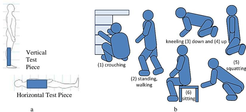
Figure 3 – (a) Portions of humans that the current standard test pieces may represent. (b) Examples of various human poses not represented by the test pieces.
