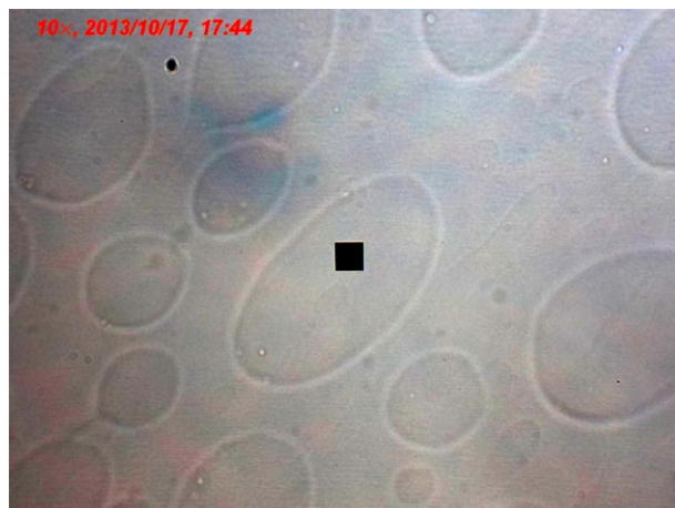
FIGURE 13.15 Image of cellulosic nanomaterials in an aqueous solution on a quartz slide under a quartz cover slip. The black square in the center is the entrance aperture of the MSP. The aperture is 12\ \mu\text{m} \times 12\ \mu\text{m} .
