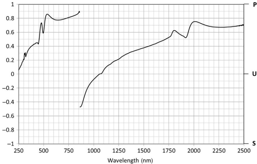
FIGURE 5.2 Degree of polarization (\Phi_p - \Phi_s)/(\Phi_p + \Phi_s) , where \Phi_p and \Phi_s are the radiant flux in p- and s-polarization, respectively, as function of the wavelength for a typical double monochromator UV/Vis/NIR spectrophotometer.
