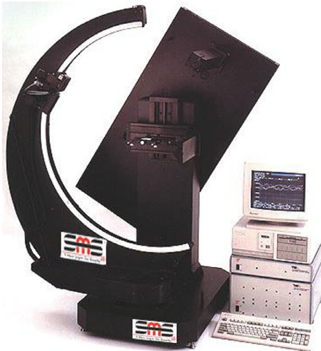
FIGURE 8.8 The TASC scatterometer is capable of reflective and transmissive measurements over the full hemisphere, while keeping the sample horizontal. Used with permission.
