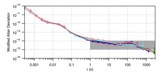
FIG. 9. (Color online) Modified Allan deviation. Multiple measurements are shown for the 2-km path to show the similarity between measurements (triangles). The shaded region represents the limit set on the accuracy by temperature drifts of 0.5 to 5  $^{\circ}$ C/h or platform motion of 1 mm/h to 1 cm/h.
