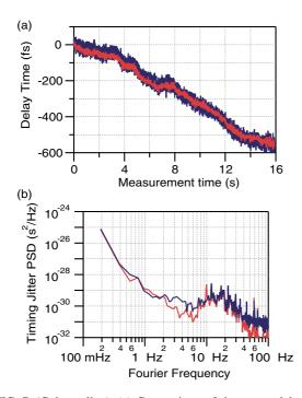
FIG. 7. (Color online) (a) Comparison of the group delay, blue (dark gray), and carrier-phase delay, red (light gray), for a low-turbulence period with few, or no, carrier-phase phase slips. (b) Corresponding PSD for the group and carrier delays. The increase below 10 Hz is due to variations in the fiber-optic path length, as in Fig. 4.
