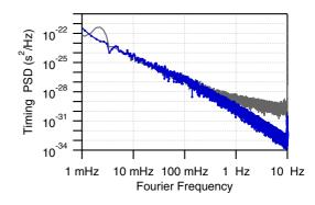
FIG. 8. (Color online) Angle-of-arrival PSD scaled as  $(2\pi cf/V)^{-2}S_{\alpha}(f)$ , blue (dark gray) line, with V = 0.7 m/s. From Eq. (2.7), this scaled PSD should overlap the time-of-flight PSD, light gray line, which it does, except where the fiber-path noise dominates at 2 mHz and above 0.5 Hz.
