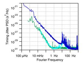
FIG. 4. (Color online) Power spectral density of timing jitter,  $S_{\text{jitter}}(f)$ , in the pulse time of flight across the entire path comprising 2 km of air and 500 m of fiber from 100  $\mu$ Hz to 1 kHz, dark blue (dark gray), as well as the contribution only from the 500 m of fiber path from building vibration–induced noise, light blue (light gray), and laboratory temperature cycling, green (medium gray).
