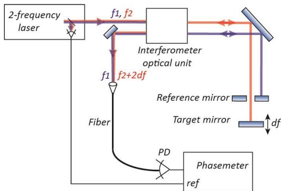
**Figure 3:** Agilent vibrometer system configuration.  $f_1$ ,  $f_2$  indicate the frequencies of the probe and reference beams, and  $df$  indicates the frequency shift due to the target mirror motion. PD: photodetector
