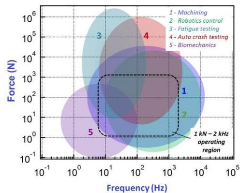
Figure 1. 1 kN, 2 kHz operating range compared to typical amplitude-timescale range of some force measurement applications.
