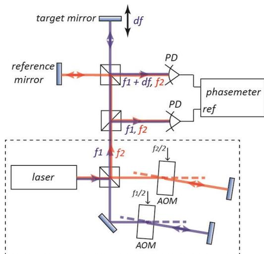
**Figure 4:** Custom auxiliary vibrometer configuration (simplified).  $f_1, f_2$  indicate the frequencies of the probe and reference beams, and  $df$  indicates the frequency shift due to the target mirror motion. Dashed line encloses heterodyne-generation section. PD: photodetector; AOM: acousto-optic modulator.
