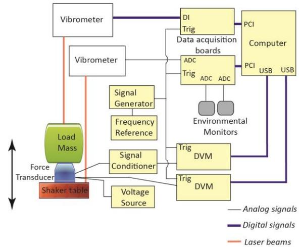
**Figure 2.** Calibration system configuration. Trig: trigger input, ADC: analog-to-digital converter, DI: digital input, PCI: PCI bus interface, USB: USB bus interface.
