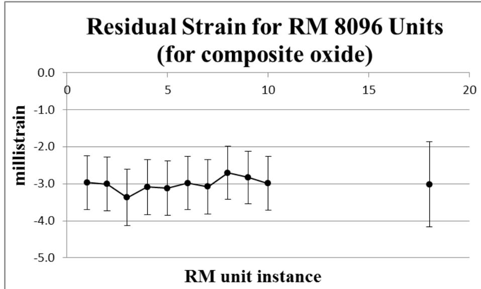
Figure 2. Residual strain values with expanded uncertainty bars,  $U_{ROI}$ , for RM 8096 units. The average value is plotted on the right with the heterogeneity expanded uncertainty (see text).
