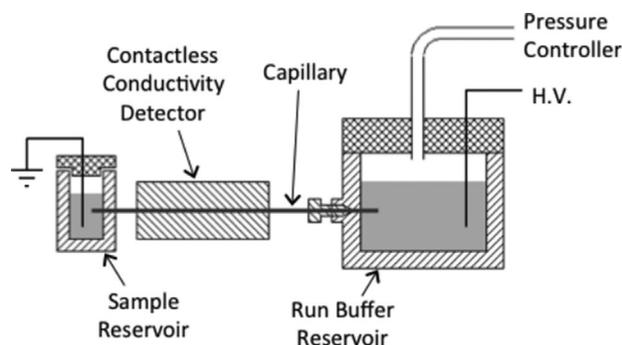
Figure 1. Schematic of GEMBE setup.
