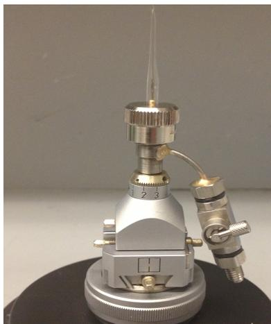
**Figure 1.** *In-situ* single crystal X-ray diffraction cell used for gas dosing experiments of  $\text{Co}_2(\text{dobdc})$
