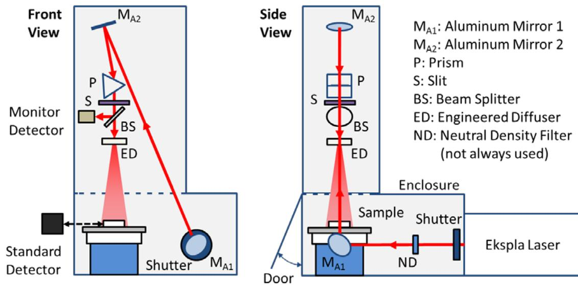
**Figure 5.** The NIST tunable UV irradiance laser system optical configuration for 210 nm to 230 nm. The dielectric mirrors are replaced by aluminum mirrors and a prism and slit are added.
