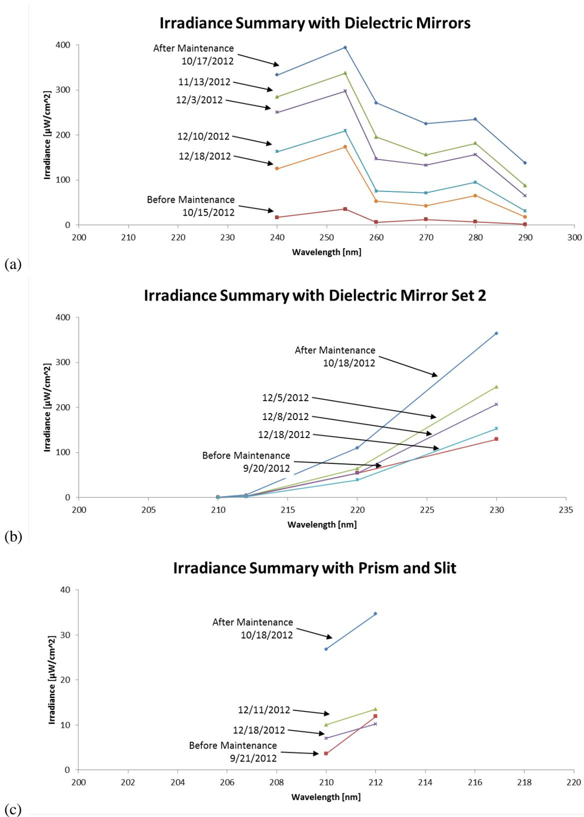
**Figure 8.** Graphs showing the decrease in irradiance ( $\mu\text{W}/\text{cm}^2$ ) over time and the improvement when some of the damaged EKSPLA laser optical components were replaced.
