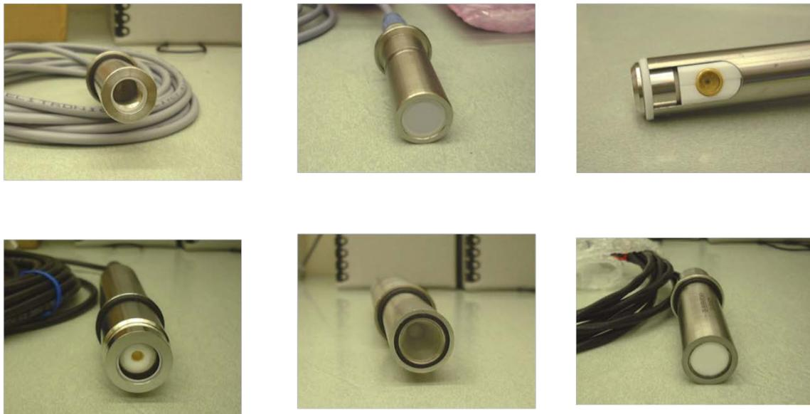
**Figure 1.** Photos of example UV sensors used in water disinfection.
