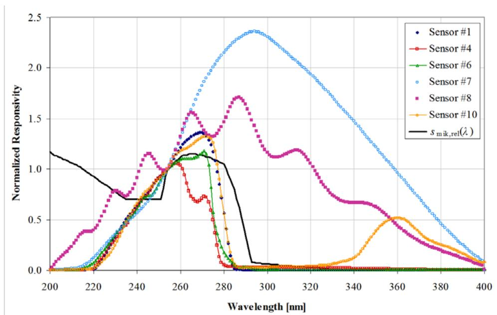
**Figure 2.** Plot of the relative spectral responsivities of six of the UV sensors measured. Also shown is the microbicidal action spectrum,  $s_{mik,rel}(\lambda)$ .
