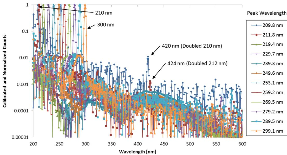
**Figure 6.** Plot of the calibrated counts normalized to the peak wavelength for the laser system spectra at the water sample position from 200 nm to 600 nm for each of the UV wavelengths of interest. The visible light has been reduced to an acceptable level.
