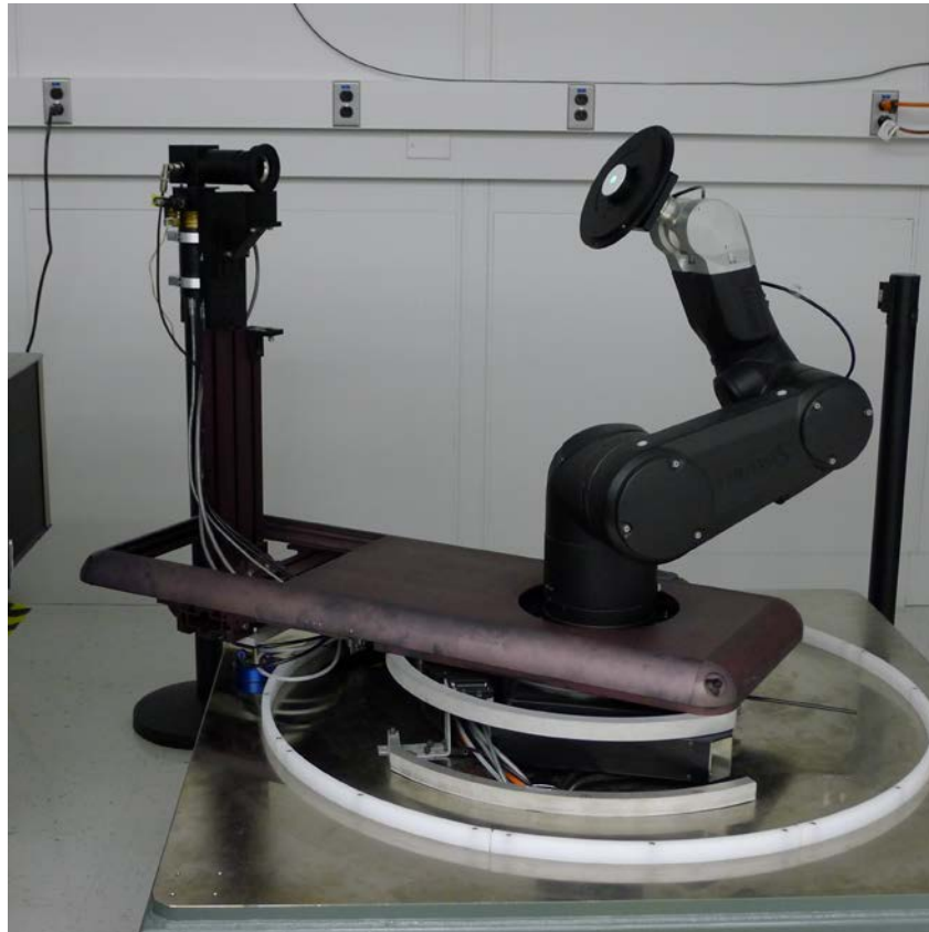
Figure 2: The Robotic Optical Scatter Instrument (ROSI) positioned for an out-of-plane scattering measurement of a white diffuse sample. Only the robotic arm sample holder and receiver are shown. The light source is on the optical table to the left and is not visible in the photo, although the illuminated area can be seen on the center of the sample.
