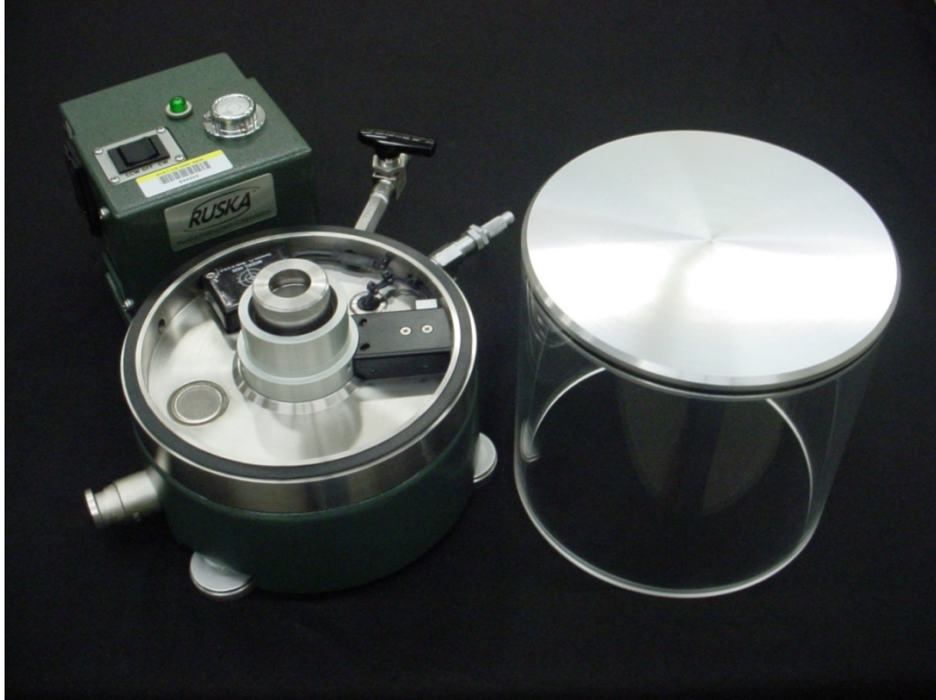
Figure 2. Ruska 2465 piston gauge base unit used in the HLPT for laboratories that do not own their own piston gauge base.
