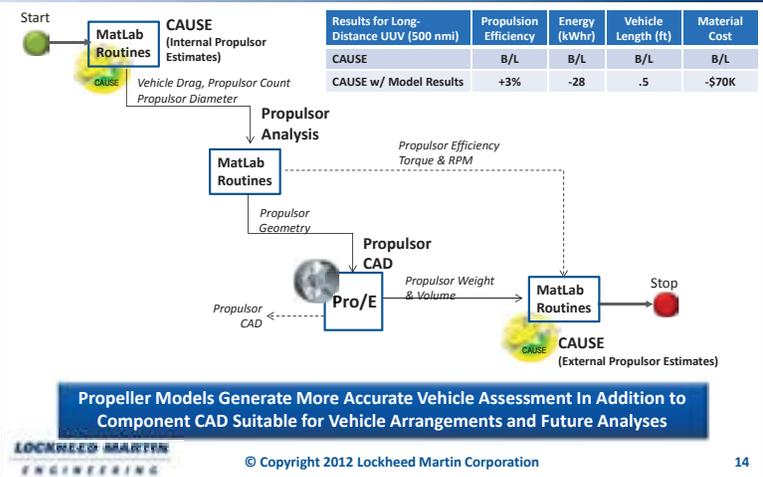
Propeller Models Generate More Accurate Vehicle Assessment In Addition to Component CAD Suitable for Vehicle Arrangements and Future Analyses
