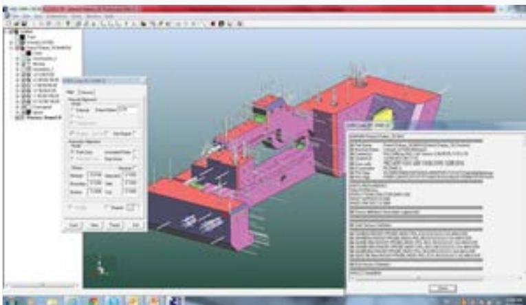
**Inspection planning & results directly from the CAD model and from any CMM machine or other inspection tools.**
