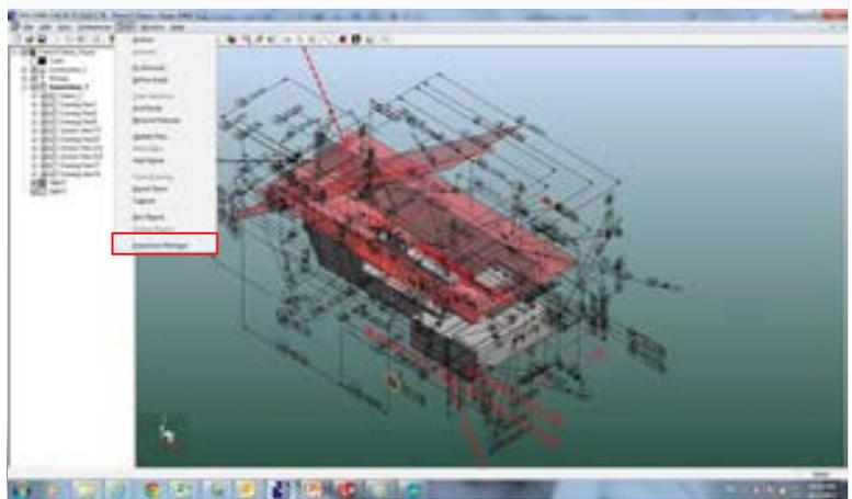
**Part inspection completed in minutes as all required information converted from the CAD model**
