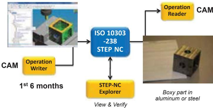
CAM to CAM data exchange for a 3 axis part
