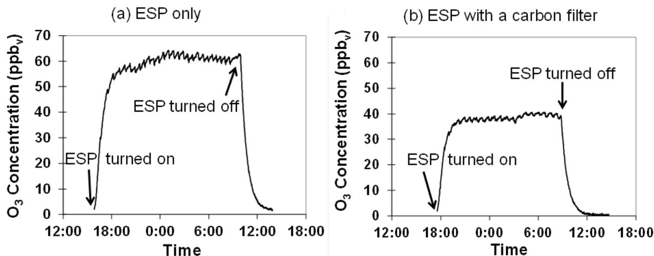
**Figure 2** Ozone concentration profile examples: (a) ESP only and (b) ESP with a carbon filter downstream – this carbon filter was one of three commercially purchased activated carbon filters, which was the most efficient filter in removing ozone among the filters tested.
