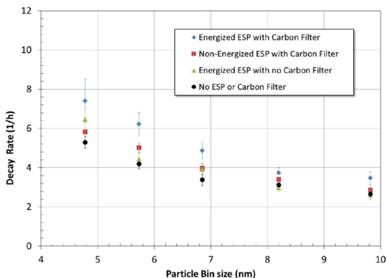
**Figure 4:** Comparison of particle decay rates for particle sizes less than 10 nm for experiments with ESP on and off. Central furnace fan was running continuously for all three cases. Error bars show the standard deviations of the averages.
