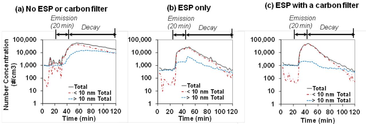
**Figure 3** Particle concentrations (a) neither ESP nor carbon filter operating (central fan off); with ESP only operating; (b) with ESP and an activate carbon media filter operating.
