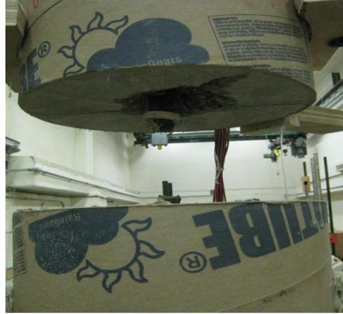
Fig. 6 – (a) No concrete damage on the free surface of the specimens with debonding; (b) cone-shaped concrete breakout on the free surface of the specimen without debonding.
