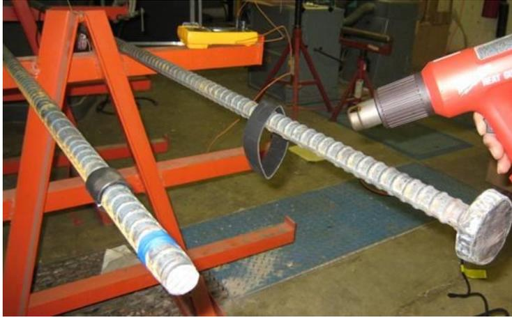
Fig. 5 – Debonding technique using polyolefin shrink tube before and after heat application.
