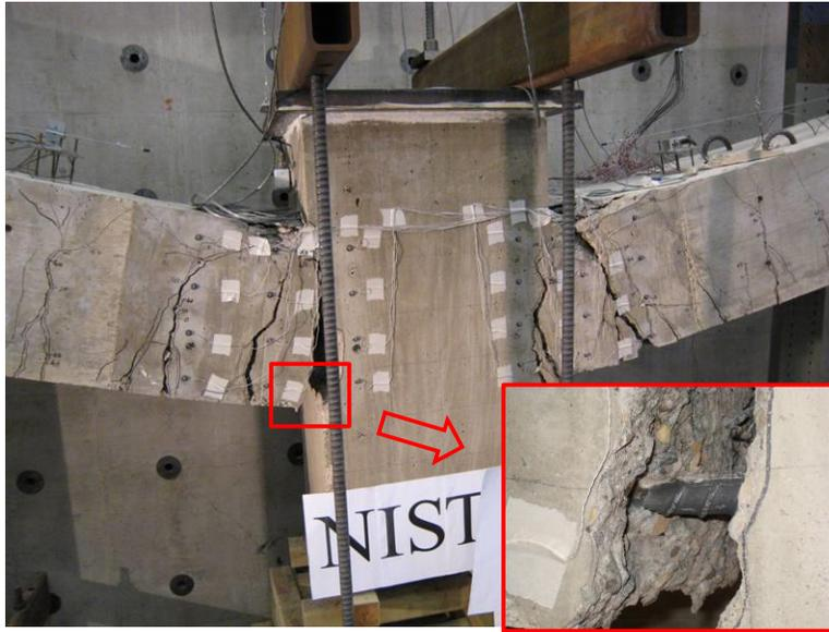
Fig. 1 – Observed reinforcing bar fracture at beam-column assembly test.
