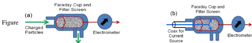
1. Charged particles (a) or known currents (b) are sourced to the Faraday cup of the aerosol electrometer.
