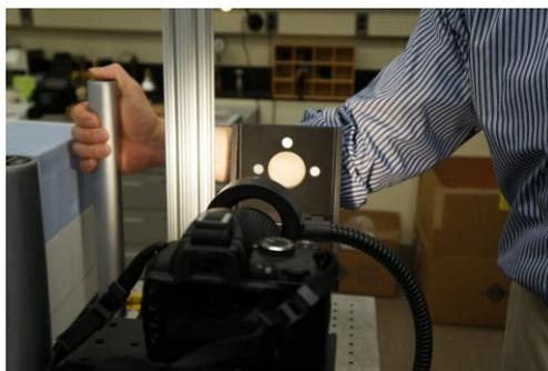
**Figure 1.** The imaging setup showing the exposed sample area of the skin. The white and grey scale references surround the aperture of the mask. The camera is positioned to view through the ring illuminator.
