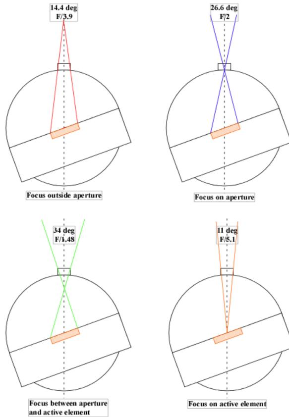
Figure 6. Schematic diagram of different beam geometries for the dome-input detector.
