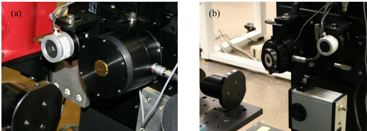
Figure 4. Photographs of dome-input pyroelectric radiometers with (a)/without dome (b) on the IRSCF.
