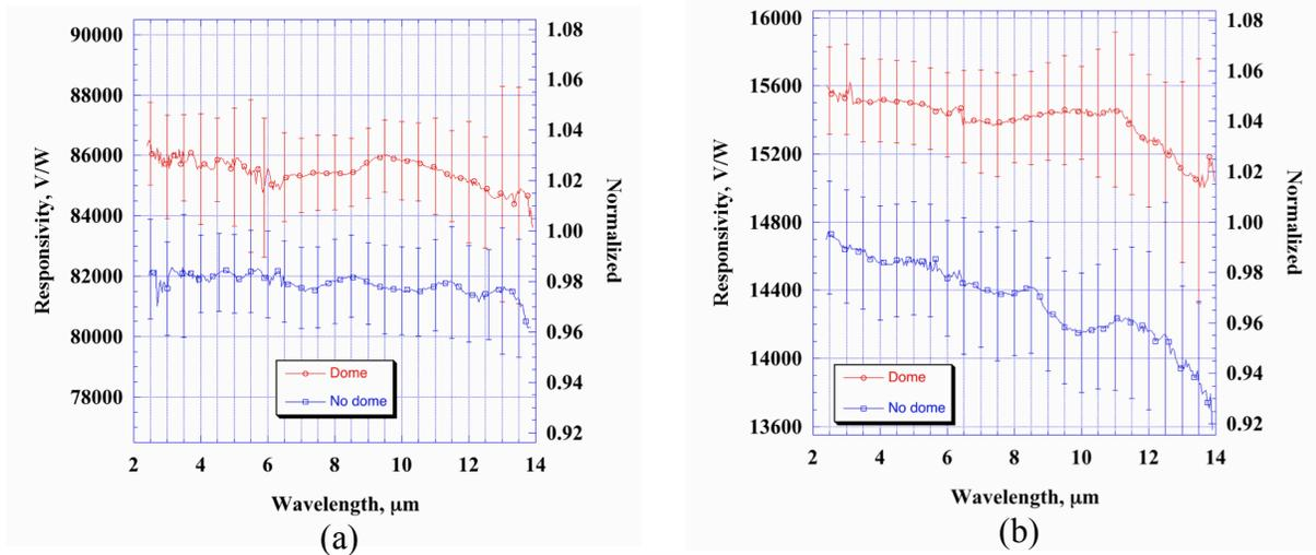
Figure 8. Comparison of spectral responsivity of two dome-input pyroelectric radiometers with 4.5 mm aperture (a) and 3.5 mm aperture (b).
