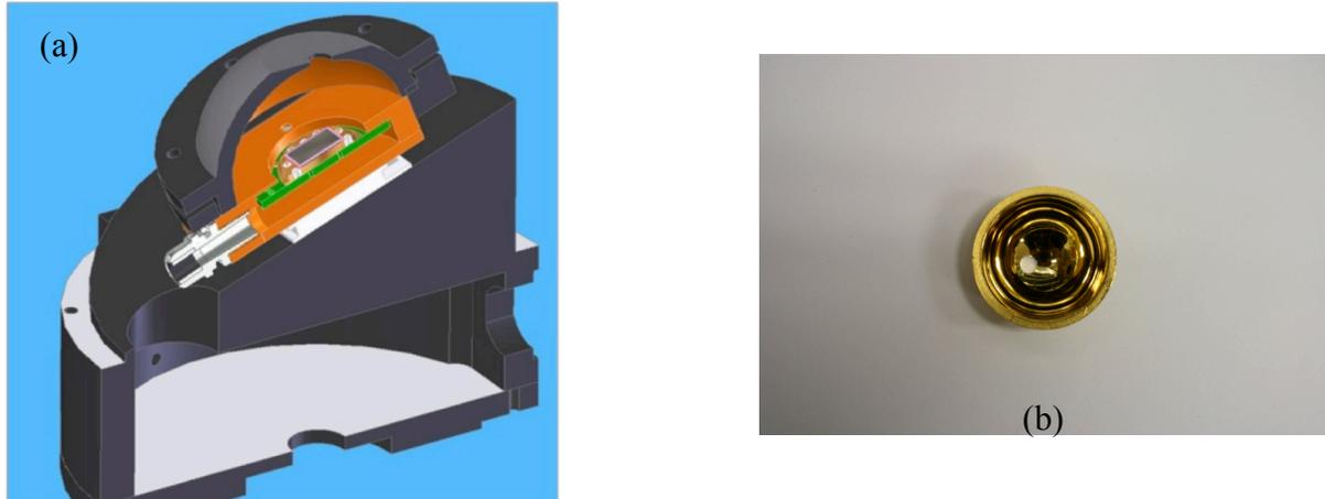
Figure 1. The cross-section of the dome-input pyroelectric radiometer head (a), and the photo of the reflective dome (b).
