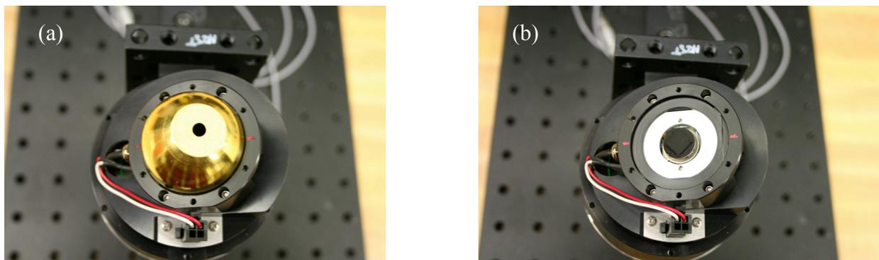
Figure 2. Photographs of the dome-input pyroelectric radiometer with (a)/ without (b) dome.
