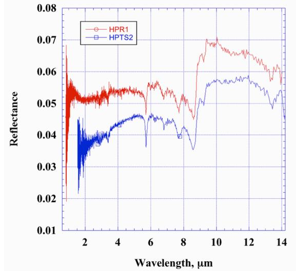
Figure 7. Results of spectral reflectance from two pyroelectric radiometers with organic black coating.
