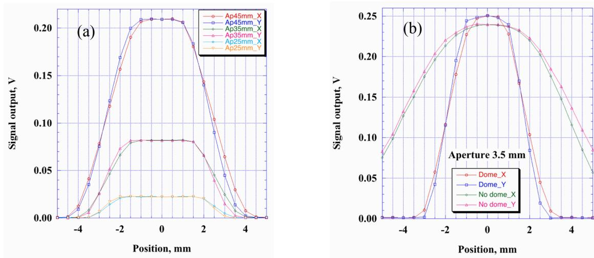
Figure 5. Spatial profiles of a standard detector at  $2.4 \mu\text{m}$  using three apertures on monochromator (a), and the spatial profiles of dome-input pyroelectric radiometer DTP3 with/without dome using an aperture of 3.5 mm on the monochromator (b).
