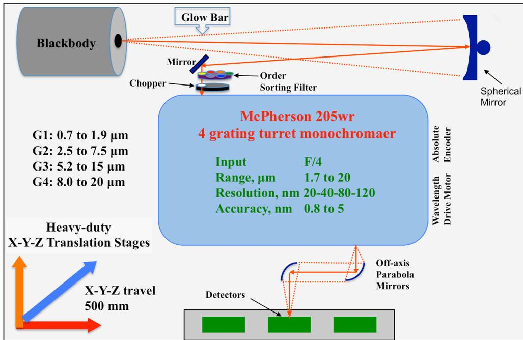
Figure 3. Schematic diagram of the IRSCF.
