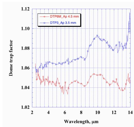
Figure 9. Comparison of light-trap efficiency of two dome-input pyroelectric radiometers.
