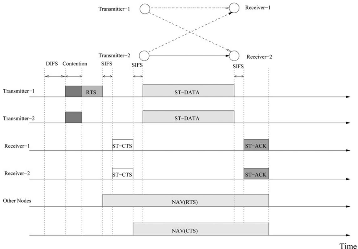
Fig. 6 MAC layer: the sequence of packet transmissions over a VMIMO link
