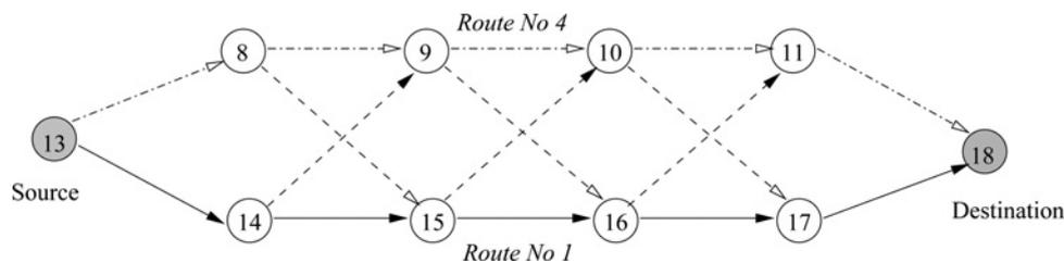
**Fig. 3** Distinctive routes that can assist the transmission of each other, which are selected using the proposed CDSR protocol for the wireless sensor network example of Fig. 2
