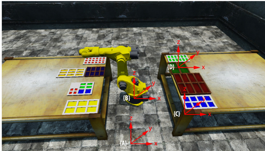
Fig. 1. A Sample of frames of reference for a kitting workstation. {A} is a frame of reference of the workstation. {B} is a frame of reference of the robotic arm in relation with {A}. {C} is a frame of reference of the worktable in relation with {A}. {D} is a frame of reference of a parts tray in relation with {C}.
