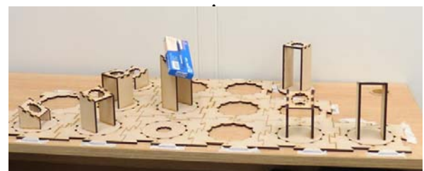
Figure 4. The GT2012 fixture with a mechanical offset configured for metrology testing.
