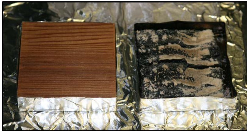
Figure 14 Photo of cedar samples before and after being burned in the cone calorimeter.
