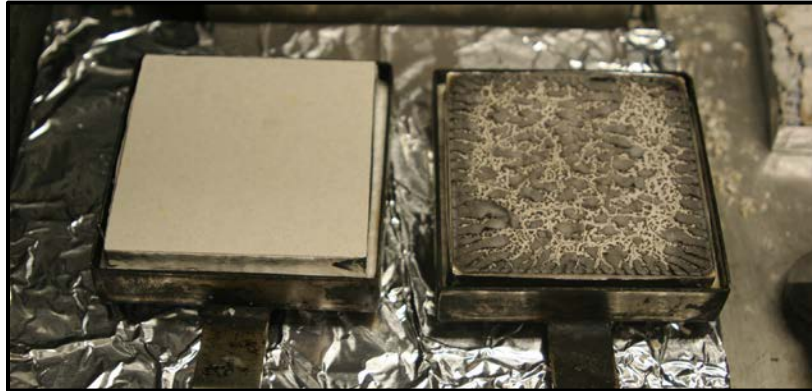
Figure 22 Photo of gypsum board samples before and after being burned in the cone calorimeter.
