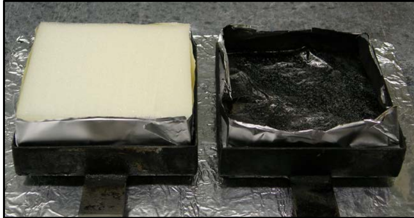
Figure 26 Photo of polyurethane foam samples before and after being burned in the cone calorimeter.
