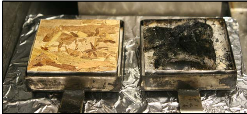
Figure 18 Photo of OSB samples before and after being burned in the cone calorimeter.
