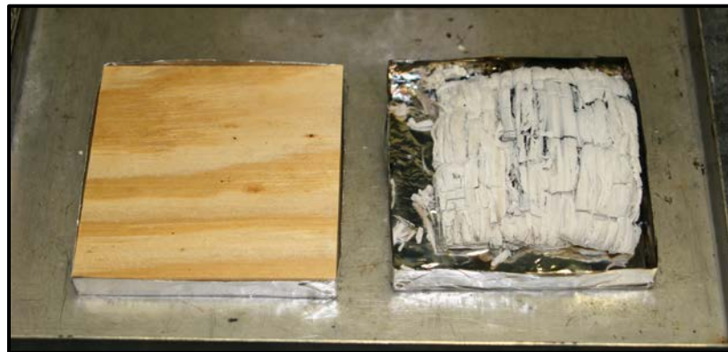
Figure 16 Photo of plywood samples before and after being burned in the cone calorimeter.
