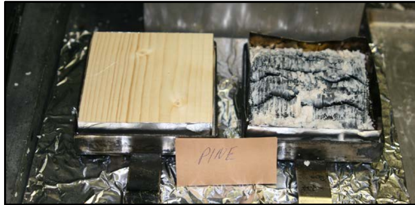
Figure 20 Photo of pine samples before and after being burned in the cone calorimeter.
