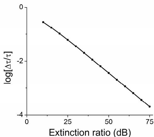
Figure 5. Calculated relative bias in measured  $\tau$  caused by fitting a single exponential function to a bi-exponential decay signal according to Eq. 1. The calculations correspond to a fitting window of approximately  $5\tau$ .
