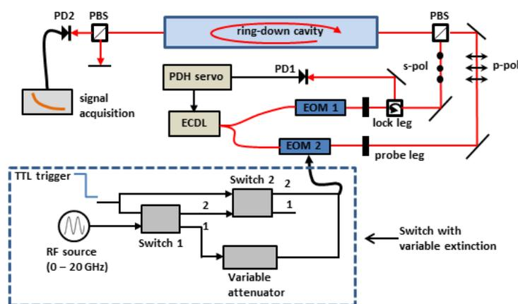
Figure 2. Schematic of the Pound-Drever-Hall (PDH) locked, FARS-CRDS spectrometer. A microwave switch with variable extinction was constructed in order to quantify the effects of finite extinction on the instrument's sensitivity. The shown components include photodiodes (PD1, PD2), polarizing beam splitters (PBS), external-cavity diode laser (ECDL), and fiber waveguide-based electro-optic phase modulators (EOM1, EOM2).
