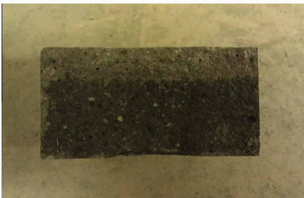
Fig. 2. A sample from the rapid chloride migration (RCM) test that was split and sprayed with silver nitrate ( \text{AgNO}_3 ).
