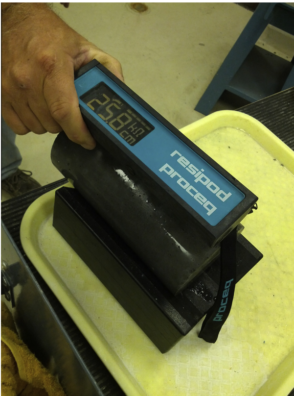
Fig. 4. Wenner probe surface testing device. Certain commercial products are identified in this paper to specify the materials used and procedures employed. In no case does such identification imply endorsement or recommendation by the National Institute of Standards and Technology, EMPA, Purdue University or Universidad del Desarrollo, nor does it indicate that the products are necessarily the best available for the purpose.
