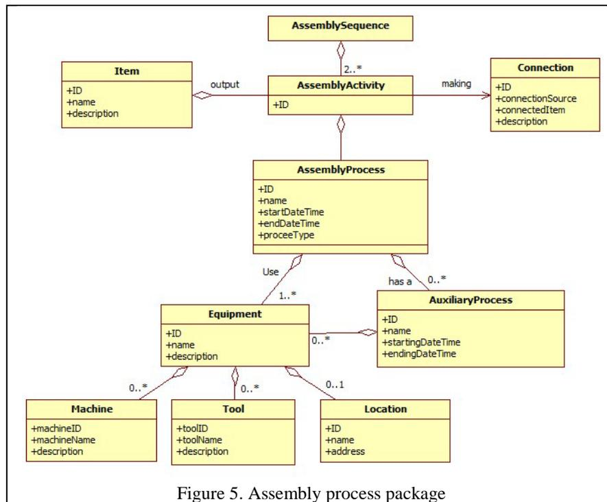
Figure 5. Assembly process package
