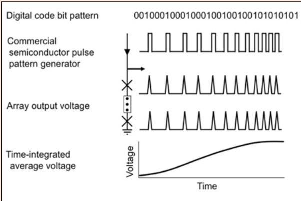
**Figure 2.** Operation of ACJVS, showing the digital code pattern produced by the code generator, the output voltage pulses of a Josephson array, and the time-average output sinusoid.
