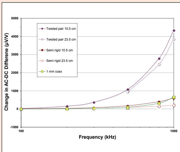
**Figure 7.** Effect of liquid helium level on transmission line error. The error bars are smaller than the markers. The errors at frequencies less than 100 kHz are negligible. The 1 mm coaxial line was measured only at the 10.5 cm level.
