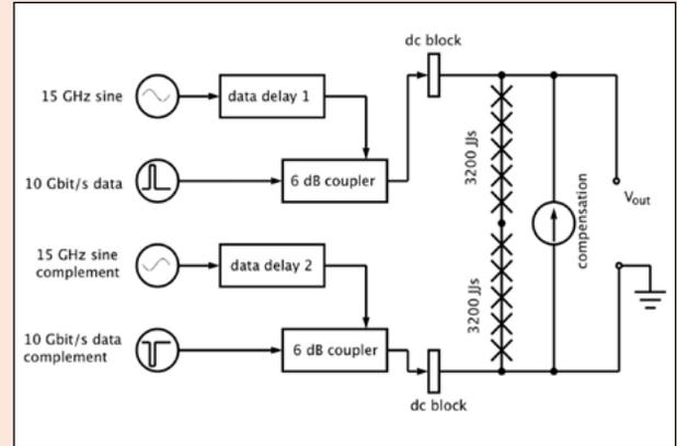
**Figure 3.** Schematic of ACJVS system showing microwave drives and pulse generators for both channels.
