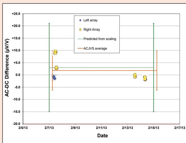
**Figure 8.** Performance of ACJVS, showing data for the right and left arrays on different dates, relative to the values predicted for the TTS from traditional scaling techniques at 50 kHz with 100 mV applied to the 220 mV range of the TTS.
