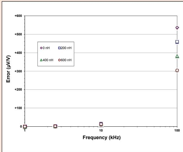
**Figure 6.** Effect of various on-chip inductances on transmission line error. The markers cover the uncertainty bars.
