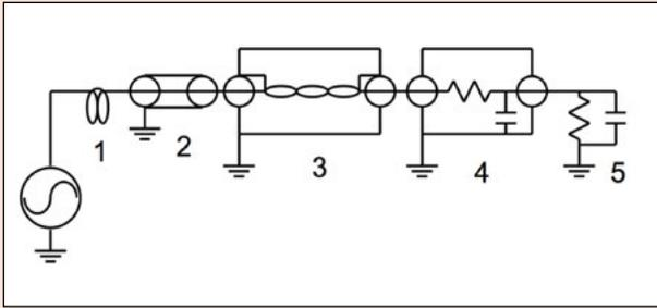
**Figure 5.** Equivalent circuit of ACJVS transmission line and TTS input showing on-chip inductances (1), 30.5 cm RG-58 cable (2), coaxial choke (3), RC filter (4) and TTS input (5).
