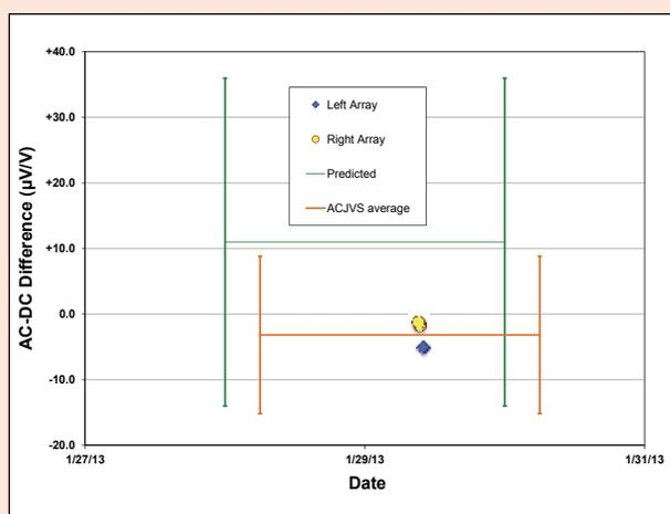
**Figure 9.** Performance of ACJVS, showing data for the right and left arrays on different dates, relative to the values predicted for the TTS from traditional scaling techniques at 100 kHz with 100 mV applied to the 220 mV range of the TTS.
