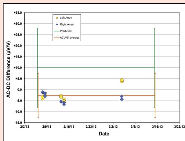
**Figure 10.** Performance of ACJVS, showing data for the right and left arrays on different dates, relative to the values predicted for the TTS from traditional scaling techniques at 50 kHz with 60 mV applied to the 220 mV range of the TTS.
