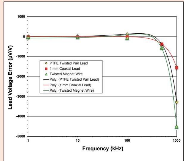
**Figure 4.** Comparison of the various types of wire used for the ACJVS output transmission line.
