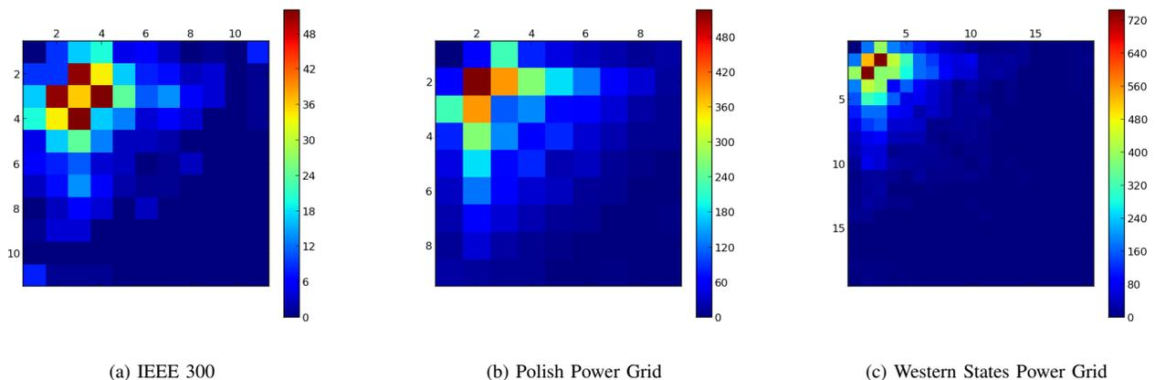
Fig. 2. This figure shows the joint degree distributions of the three test data sets. These figures show the large differences between the joint degree distributions of the three data sets. In particular, the entries  $D_{2,2}$  show radically different values between all three sets.
