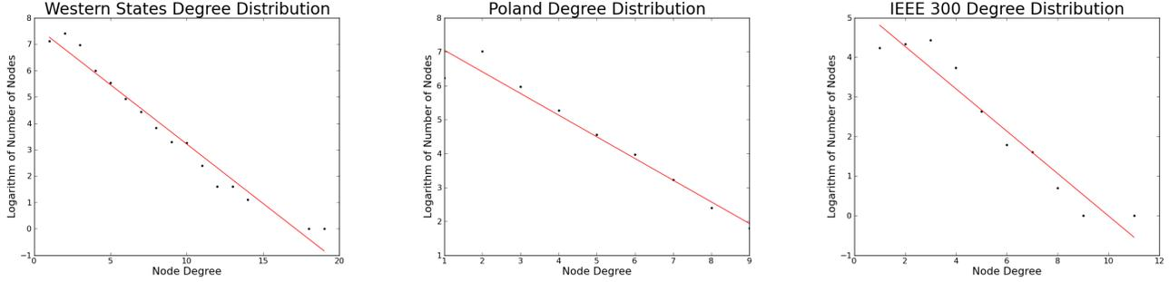
Fig. 1. A least squares fitting of the three data sets on a semi-log domain. This fitting gives support to the idea that power grid degree distribution are actually exponential distributions and not power-law.
