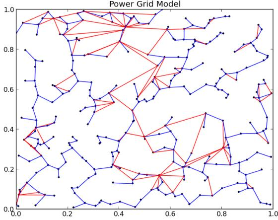
Fig. 3. This figure shows a typical model created by the algorithm. The blue edges represent those selected for the spanning while the red edges are the ones added afterwards. The size of the model was chosen to match size of the IEEE 300 data set. This model had 300 nodes, 395 edges, an average degree of 2.63, a maximum degree of 13, an average clustering coefficient of 0.16, an average path length of 13.58, and a diameter of 41.
