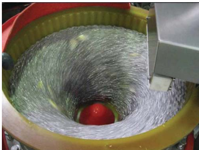
Fig. 1—Blanks are mixed with stainless steel balls and pickling compounds in a burnishing machine (color figure available online).
