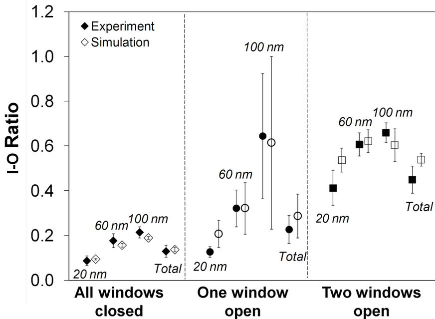
Fig 5. Indoor-outdoor (I-O) ratio for three different window operation modes: all windows closed, one window open, and two windows open. Measurement and simulation results are reported for 20 nm, 60 nm, 100 nm, and total UFP (3-100 nm). Error bars represent standard error from the mean obtained from multiple tests.
