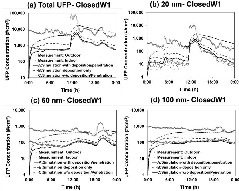
Fig 3. Time-varying particle concentration profiles – measurement vs. simulation for the test ClosedW1 for different cases of penetration and deposition: (a) Total UFP concentrations, (b) 20 nm, (c) 60 nm, and (d) 100 nm.
