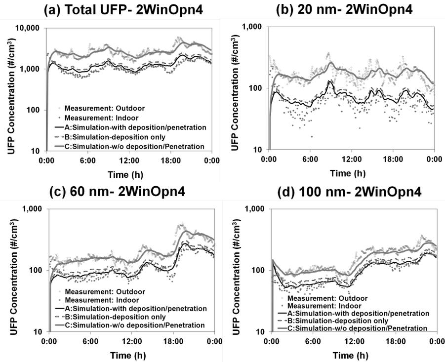
Fig 4. Time-varying (24-h) particle concentration profiles – measurement vs. simulation for the test ClosedW1: (a) Total UFP concentrations, (b) 20 nm, (c) 60 nm, and (d) 100 nm.
