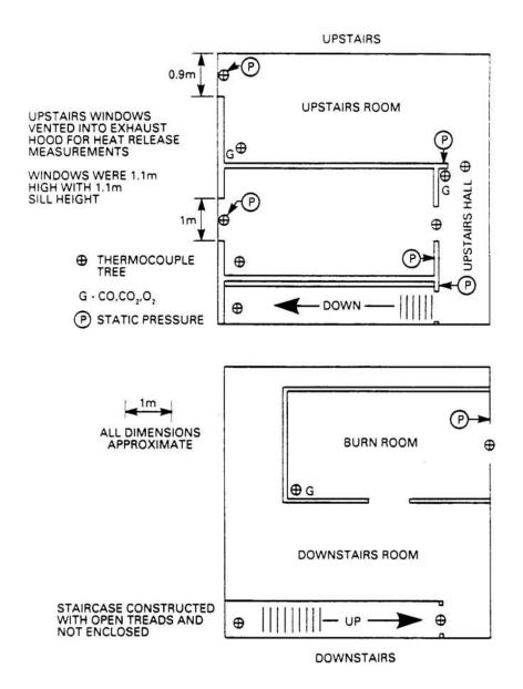
Figure 1. Layout and instrumentation of a simulated residential townhouse used for several full-size room fire tests.
