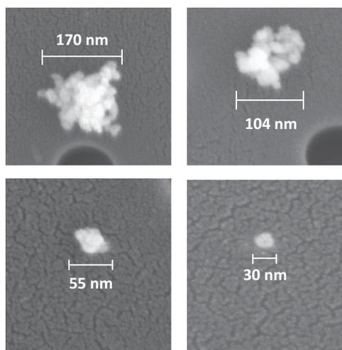
**FIGURE 5.** Scanning electron microscopy images of dry nano silver particles collected from inside the exposure chamber on a polycarbonate filter during the low dose exposure. The most commonly observed particle sizes were 30–80 nm.
