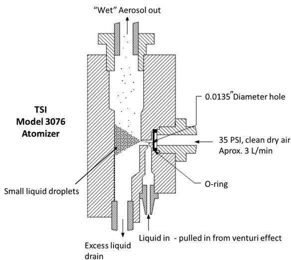
**FIGURE 2.** Diagram of the TSI 3076 aerosol generator.
