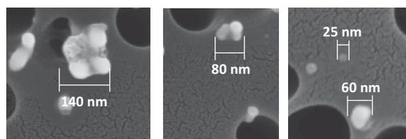
**FIGURE 6.** Scanning electron microscopy images of dry nano silver particles collected from inside the exposure chamber on a polycarbonate filter during the high dose exposure. The most commonly observed particle sizes were 30–80 nm.
