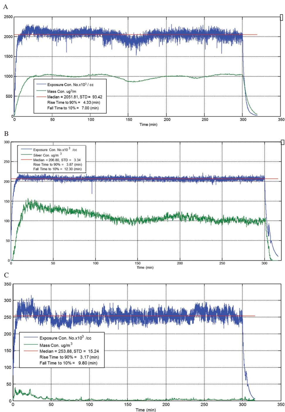
**FIGURE 3.** Exposure chamber concentration data for the high dose (NIST sample; 200 mg/L) aerosol exposure (A), the low-dose (MesoSilver sample; 20 mg/L) aerosol exposure (B), and the control (deionized water) aerosol exposure (C). Particle number ( $\times 10^3$ ) and particle mass ( $\mu\text{g}/\text{m}^3$ ) are given on the y axis (color figure available online).
