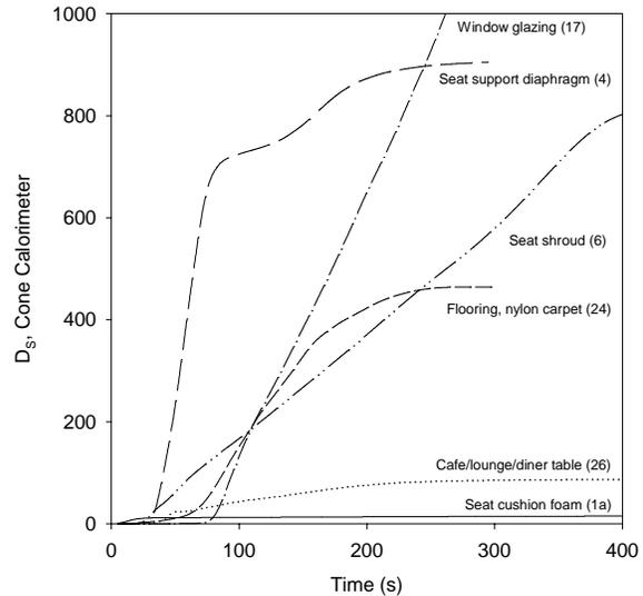
Figure 3. Specific optical density for several materials as determined from the specific extinction area as measured in the Cone Calorimeter.
