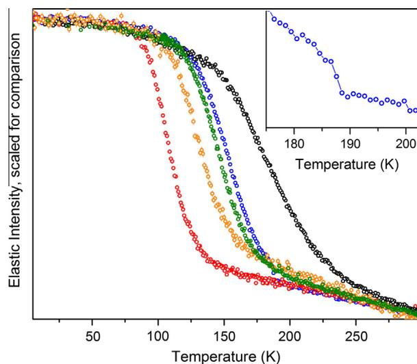
**Fig. 2.** Fixed-window scans for  $\text{BH}_4^-$  anions in  $\text{MBH}_4$  compounds (from right to left,  $M = \text{Li, Na, K, Rb, and Cs}$ ) as a function of temperature. The inset shows FWS evidence of the order–disorder phase transition of  $\text{NaBH}_4$  just below 190 K.
