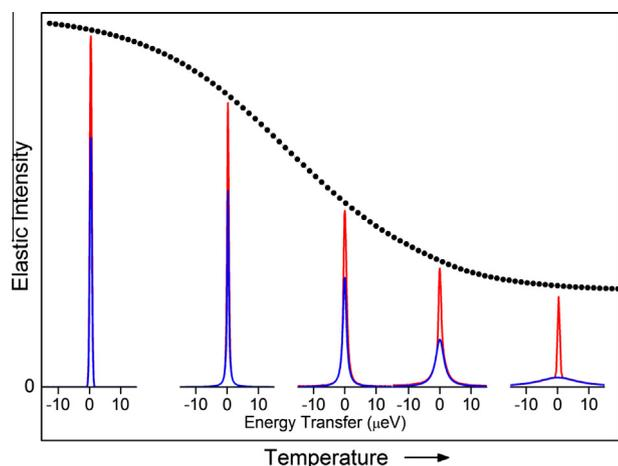
**Fig. 1.** A typical fixed-window scan at zero energy transfer (closed circles), showing the effect of the temperature-dependent broadening of the quasielastic component (blue line) on the overall neutron scattering spectrum (red line). (For interpretation of the references to colour in this figure legend, the reader is referred to the web version of this article.)
