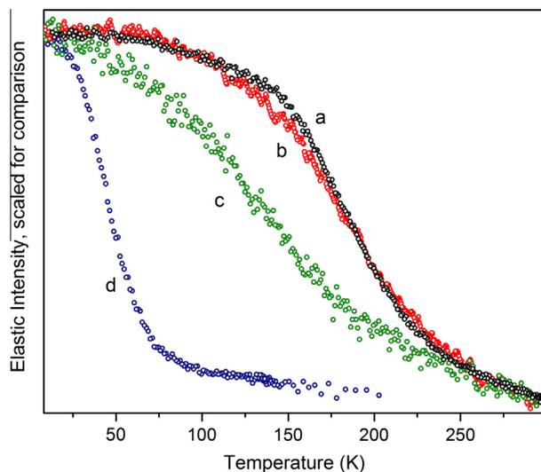
**Fig. 3.** Fixed-window scans as a function of temperature for  $\text{BH}_4^-$  anions in (a) bulk  $\text{LiBH}_4$ , (b)  $\text{LiBH}_4$  (completely filled) in a 13 nm carbon aerogel, (c)  $\text{LiBH}_4$  (partially filled, 22%) in a 13 nm carbon aerogel, and (d) a 1:1  $\text{LiBH}_4\text{-LiI}$  solid solution.
