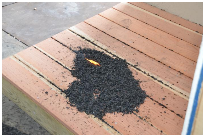
Figure 8 Flaming ignition of Redwood decking assembly.
