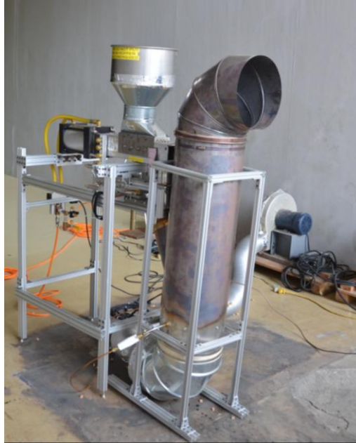
Figure 1 Full-scale continuous Feed Firebrand Generator installed in BRI's FRWTF. The device was not producing firebrands at the time of this photograph.
