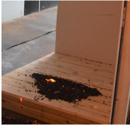
Figure 7 Flaming ignition of Douglas-Fir decking assembly
