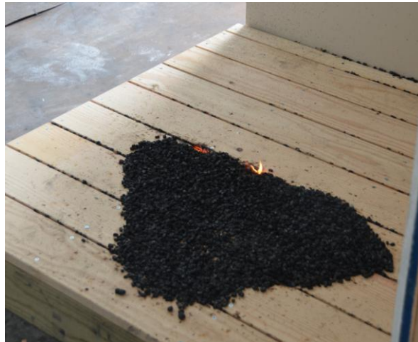
Figure 8 Flaming ignition of Redwood decking assembly.
