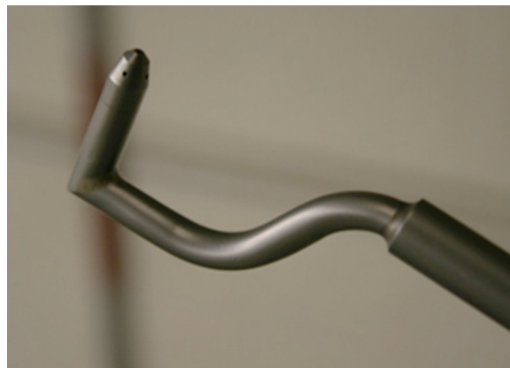
Fig. 1. Cone-shaped, five-hole Pitot tube. The diameter of the curved tube is 9.5 mm.
