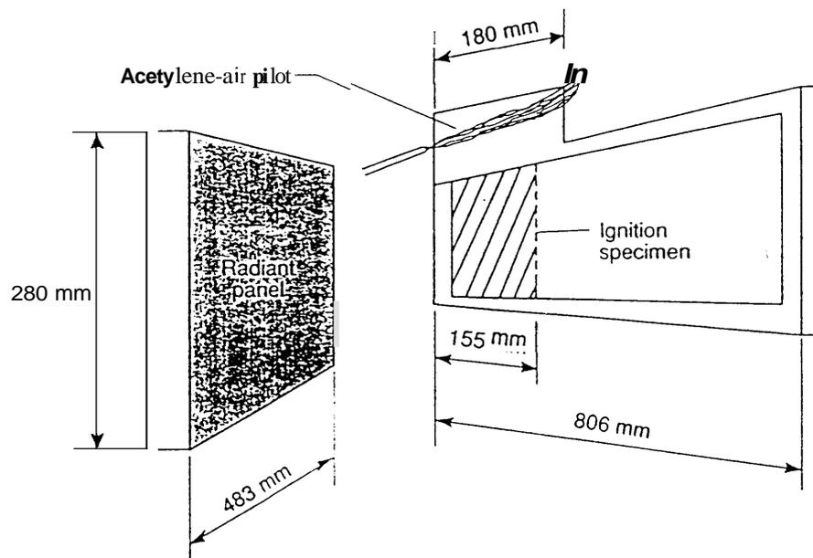
Figure 1. Schematic of LIFT apparatus.
