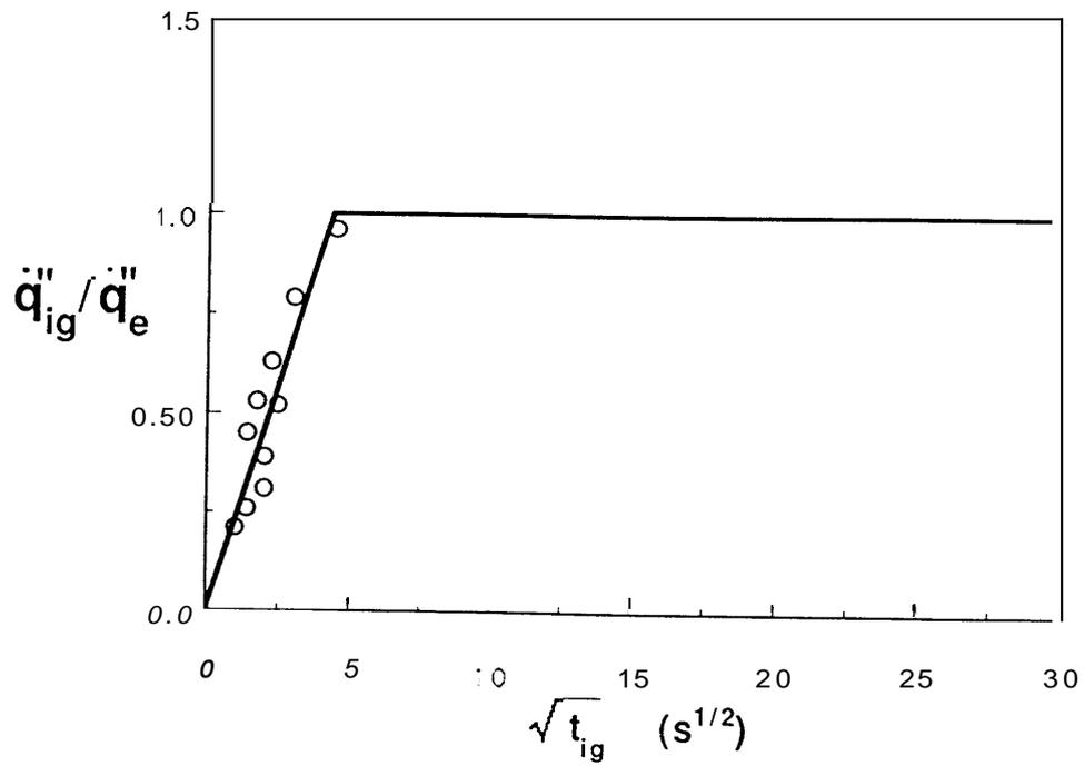
Figure 2. ignition data correlation for rigid polyurethane panel foam
