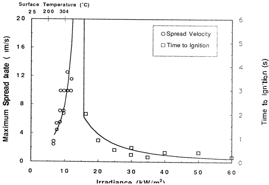
Figure 4. Spread and ignition results for rigid polyurethane panel foam.
