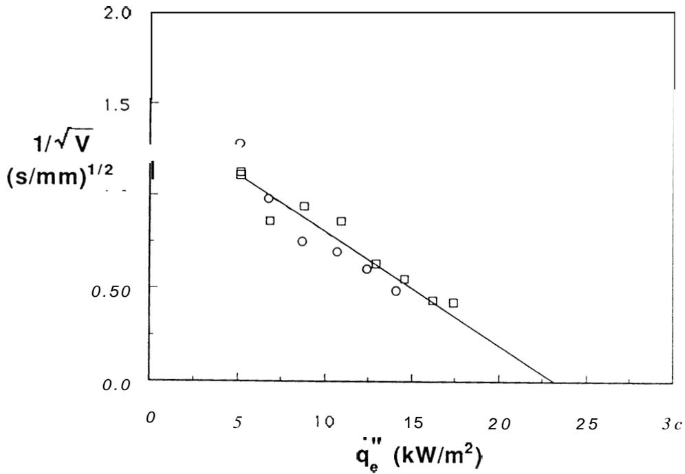
Figure 3. Lateral flame spread correlation for rigid polyurethane foam (spray).
