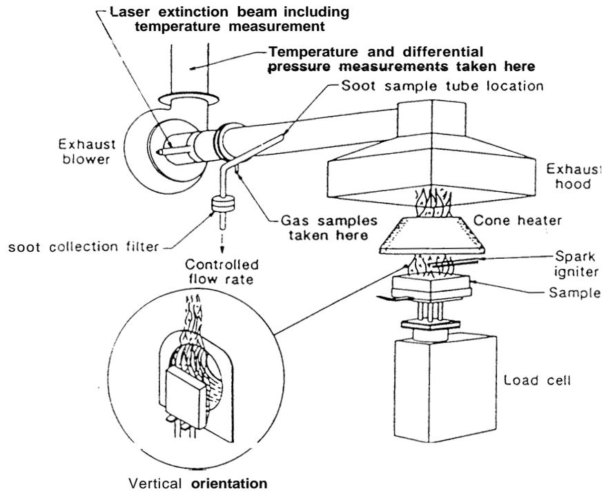
**Figure 9. Schematic of the Cone Calorimeter**
