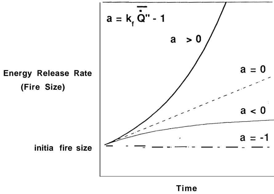
Figure 5. Dependence of  $a$  on the fire growth potential.
