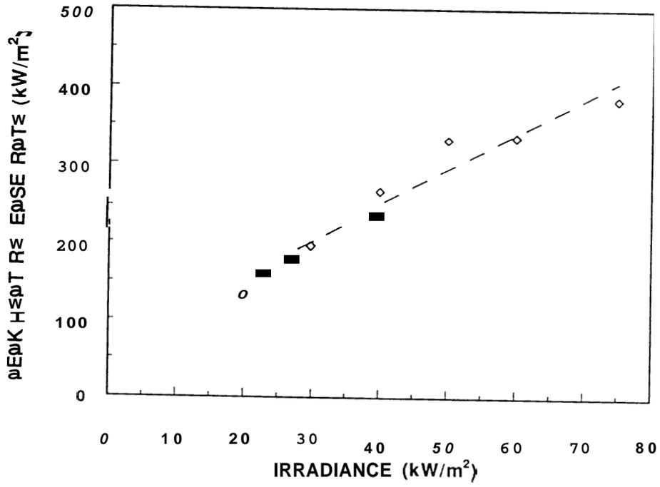
Figure 11. Peak rate of heat release versus irradiance for rigid polyurethane foam (spray).
