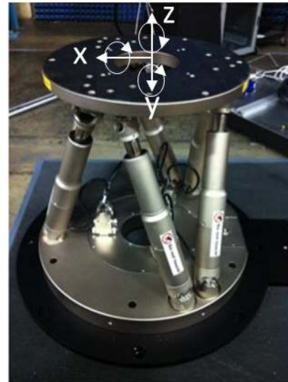
Figure 4 – Six-Axes Parallel Kinematic Hexapod Robot
