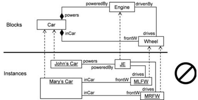
Figure 11. Antiexample for assembling components.
