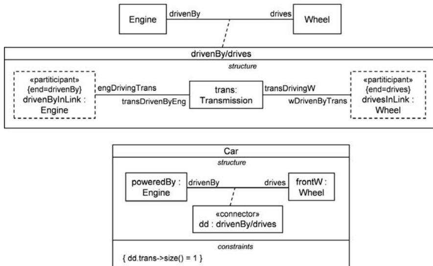
Figure 15. Association blocks with internal structure.
