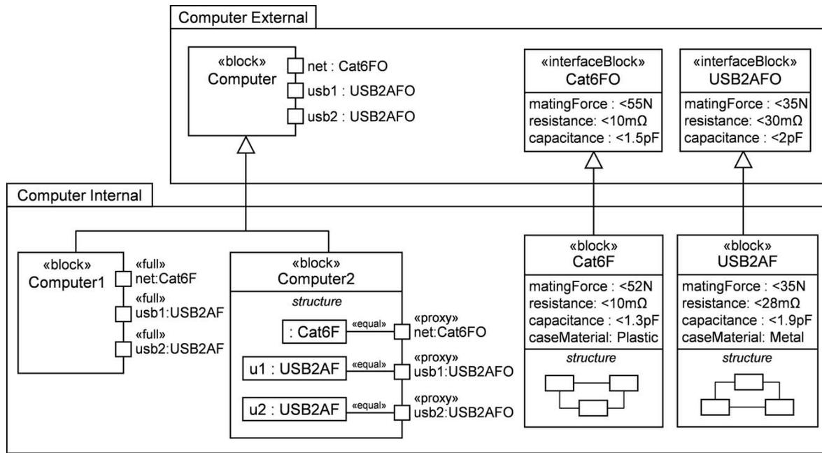
Figure 21. Full ports and proxy ports.
