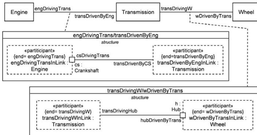
Figure 19. Incremental association decomposition with ports.
