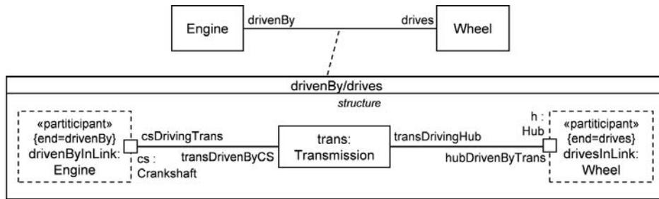
Figure 18. Association decomposition with ports.
