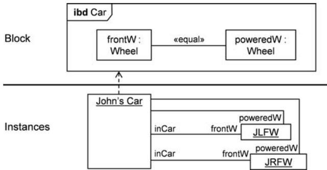
Figure 16. Binding connectors.
