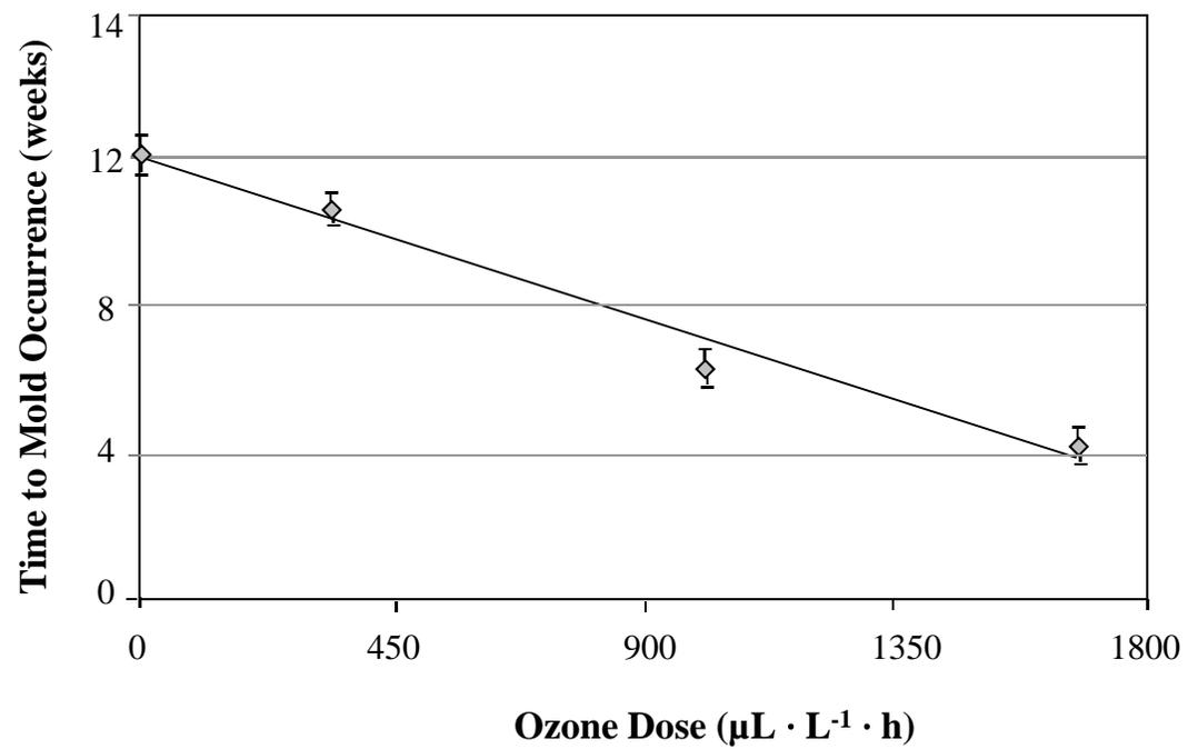
**Figure 5. Effects of ozone dose on time to mold occurrence for ozone-treated bamboo incubated at 85 % RH and 30 °C condition. The error bars represent one standard deviation.**
