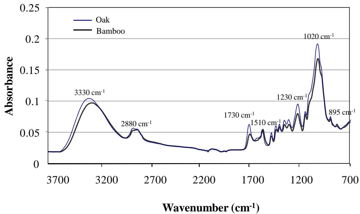
**Figure 3. ATR-FTIR spectra of untreated bamboo and untreated oak.**
