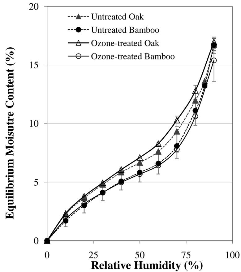
**Figure 2. Moisture sorption isotherms of bamboo and oak before and after ozonation. Symbols are experimental data and lines are best fitting curves. Error bars represent value ranges**
