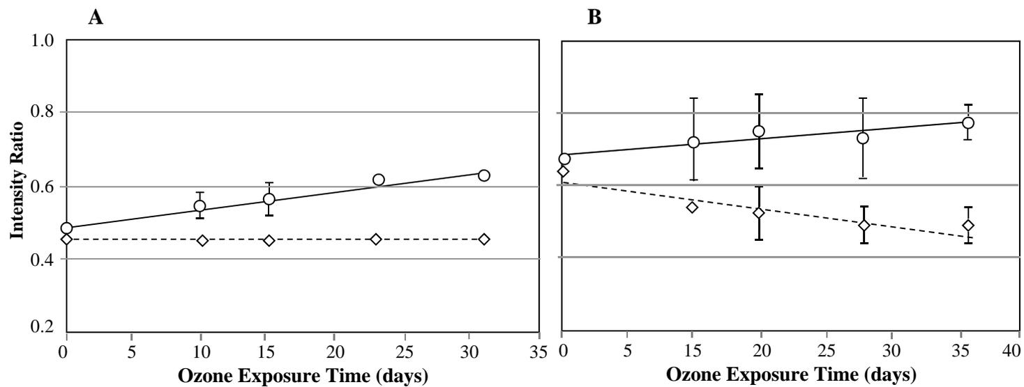
**Figure 4.** ATR-FTIR Intensity changes of the 1510 cm<sup>-1</sup> (◇) and 1730 cm<sup>-1</sup> (○) bands as a function of ozone exposure for oak (A) and bamboo (B). The intensities have been normalized to that of the 895 cm<sup>-1</sup> band. The error bars represent one standard deviation.
