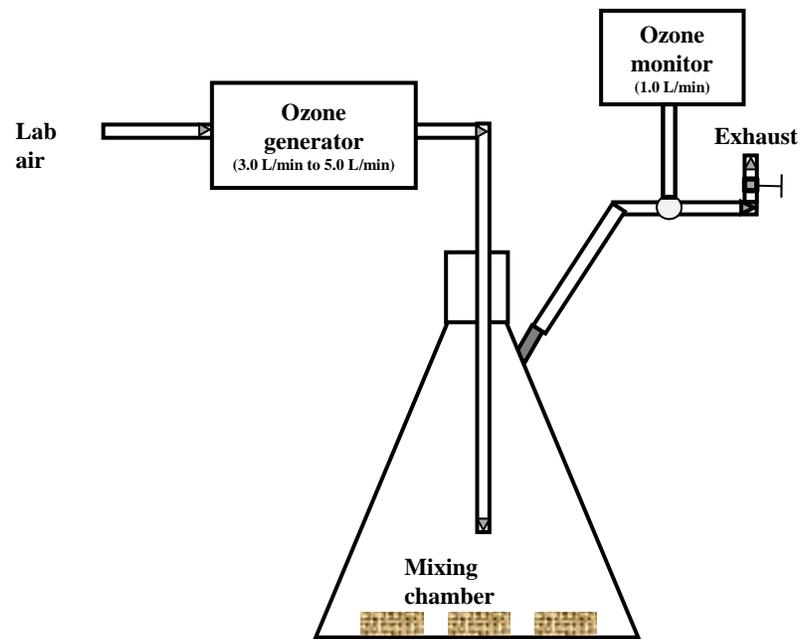
**Figure 1. Experimental apparatus for ozone treatment of bamboo and oak samples.**
